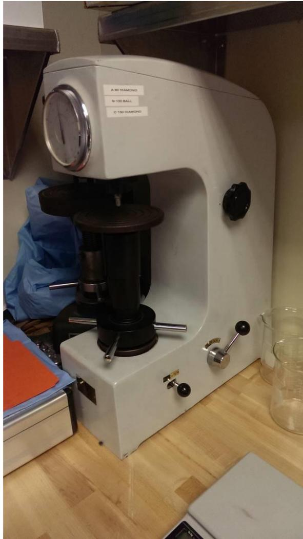
**Figure 24. Rockwell Hardness Tester**
