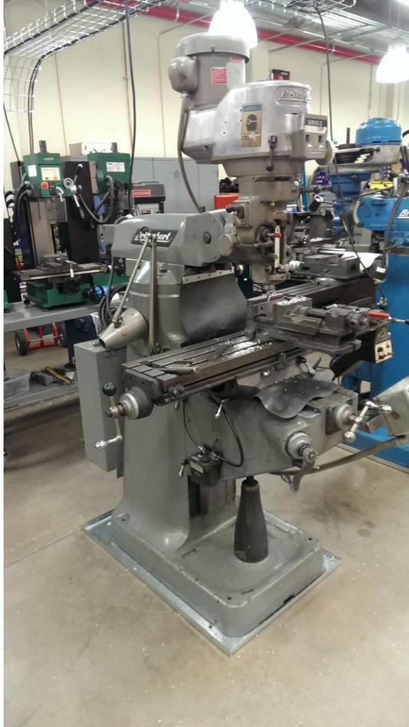
**Figure 21. Bridgeport Vertical Milling Machine**
