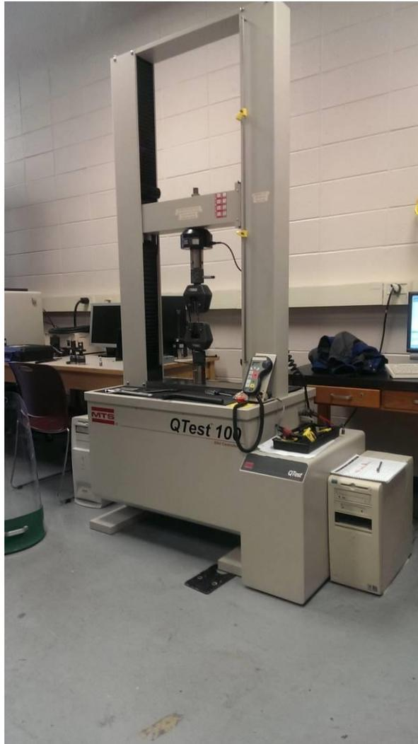
**Figure 25. MTS Q Test 100 Tensile Tester**
