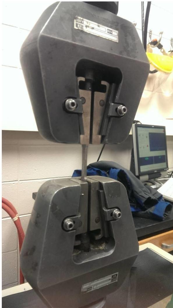
**Figure 26. Tensile Testing Jaws with Specimen Inserted**
