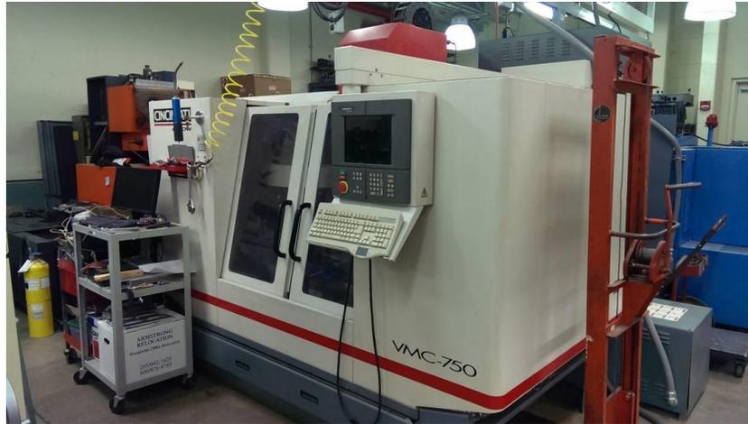
**Figure 20. Cincinnati Arrow VMC 750 CNC Mill**
