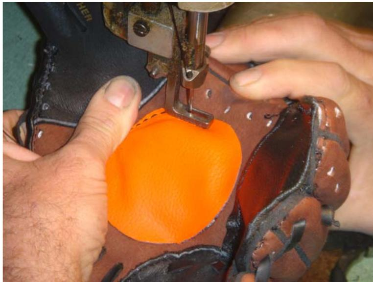
Figure 45- Construction: Center Target
