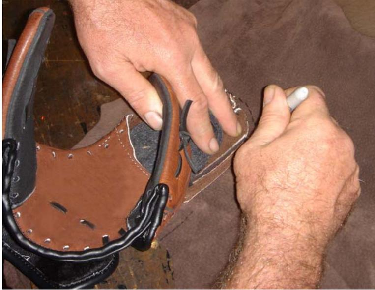
Figure 43- Construction: Making of the Pattern
