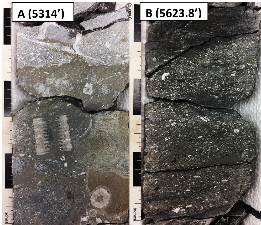
Figure 25: Core photographs of the bioclast-lithoclast wackestones-floatstone lithofacies. Scale is in inches. (A) Bioclast-lithoclast wackestones-floatstone comprised of skeletal fragments (crinoid ossicles) (5314.5'). (B) Bioclast-lithoclast wackestone-floatstone composed of poorly-sorted, ungraded, skeletal debris of crinoids and unidentifiable skeletal fragments and elongate mud lithoclasts (5623.8').
