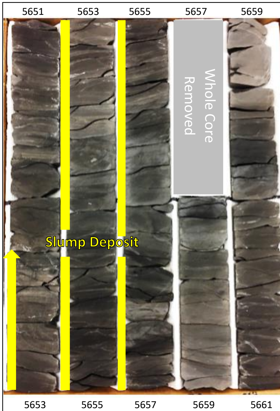
Figure 12: Photograph of core interval 5651'-5661' displaying a slump deposit comprised of contorted siltstone beds.
