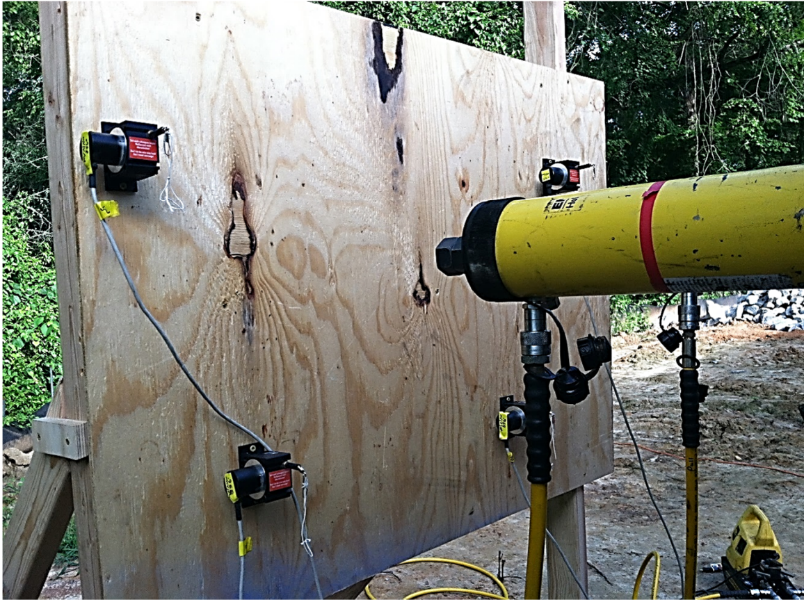
Figure 4-8 – Wire Pot Deflection Measurement Devices prior to Load Testing
