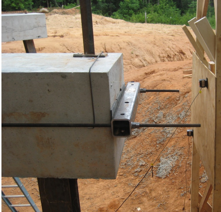
Figure 4-48 – High Strength Threaded Rod and HSS Bearing Tube
