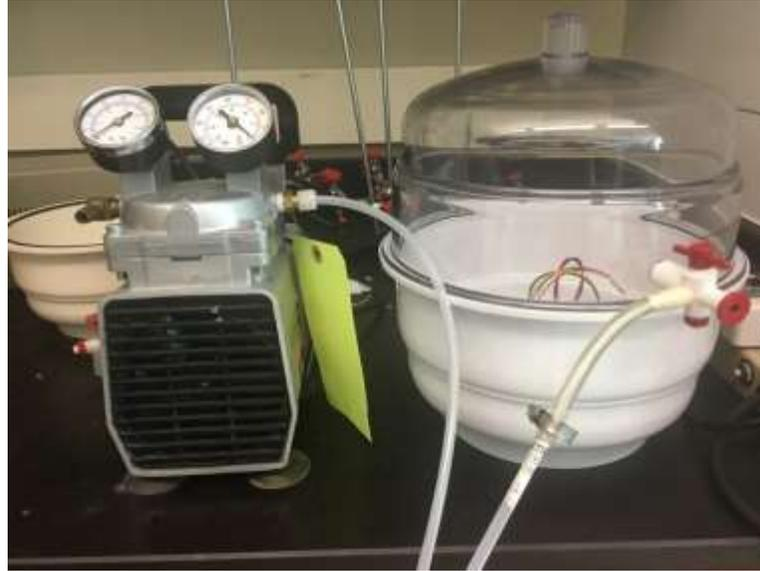
**Figure 53:- Vacuum Pump and Desiccator**
