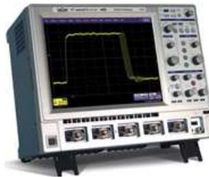
**Figure 12:- Wave-runner Xi series oscilloscope**
