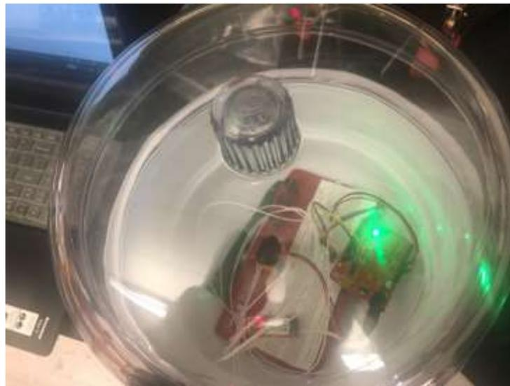
Figure 51:- Hardware test bed with MEMS test board assembly in the vacuum desiccator
