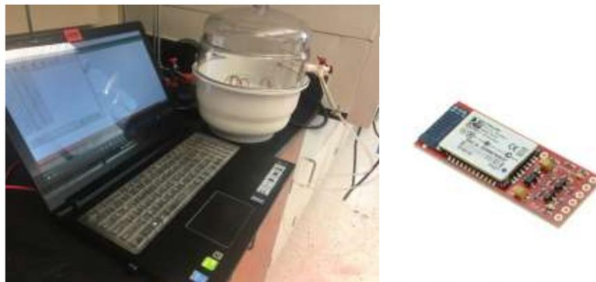
Figure 52:- Bluetooth module and USB-Bluetooth dongle connected to DAQ
