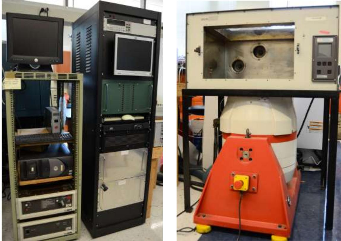
**Figure 17:- Data Acquisition System with LDS power supply (left) and Vibration-Temperature setup (right)**
