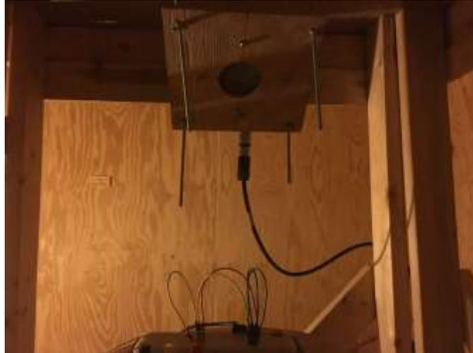
**Figure 91:- Source speaker on top of MEMS test board assembly**
