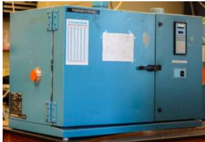
**Figure 230: - Thermal Cycling chamber for varying thermal stresses test on Li-ion batteries**
