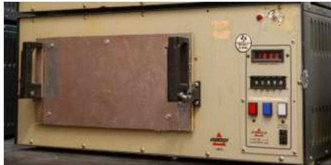
**Figure 229: - Aging oven for calendar storage of Li-ion test samples**
