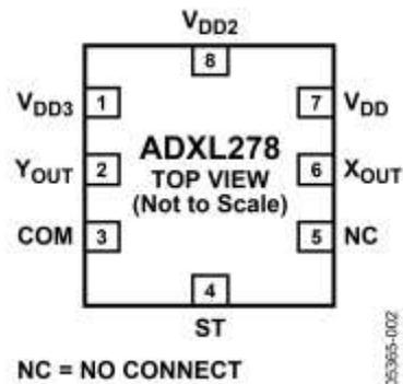
Figure 152: Layout of ADXL278, courtesy Analog devices
