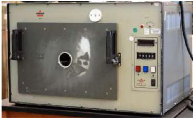
**Figure 55:- HTOL Aging Oven**
