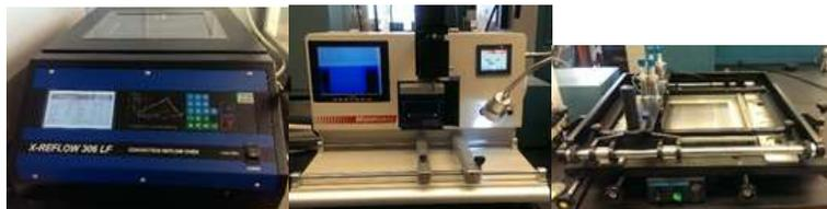
**Figure 122:- Stencil printer, Reflow oven and Pick & Place machine (CW direction)**
