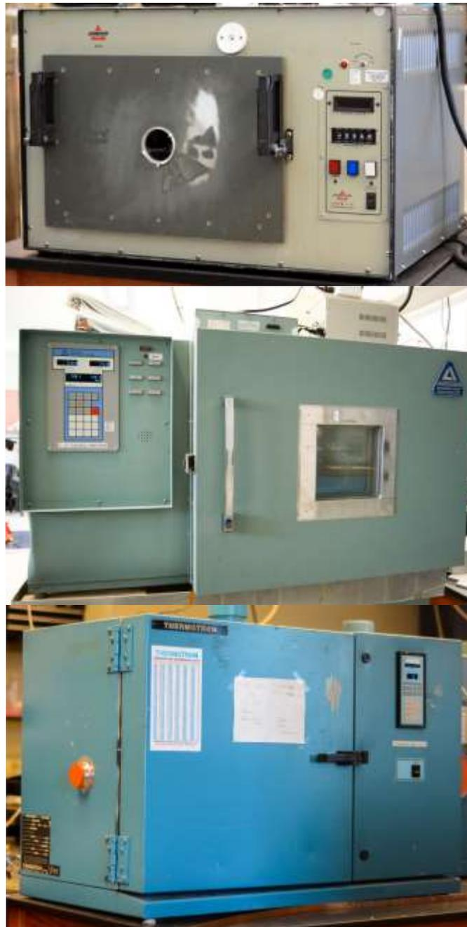
**Figure 87:- HTOL chamber (TOP), THB chamber (Middle) and LTS chamber (Bottom)**
