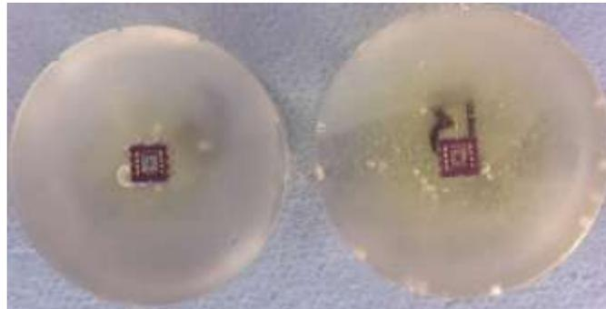
**Figure 174:** The above figure shows potted (above) and polished (below) ADXL278 samples
