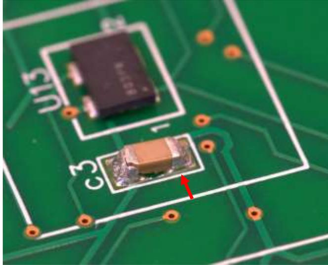
**Figure 145:- Cracked decoupling capacitor, for an 85°C/85%RH case**
