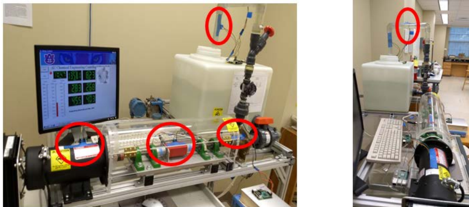
Figure 2.6 IoT enabled pump testbed (red o: IoT sensors)
