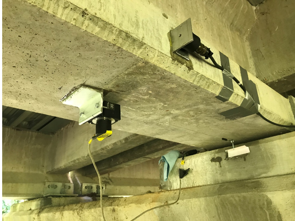
Figure 3-22 – Standard Wire Pot Set-Up
