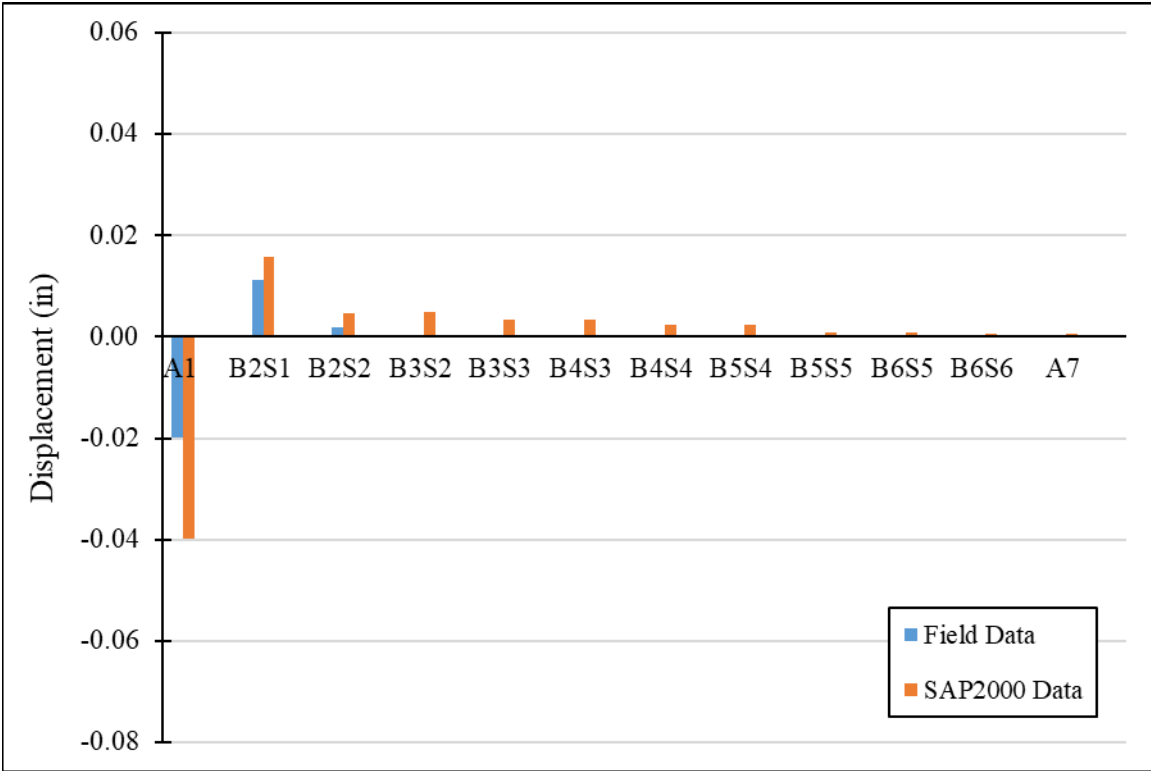
Figure 4-1 – Measured versus Model Displacements for Span 1 Static Loading
