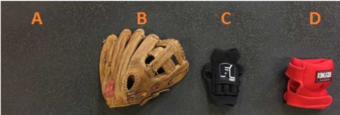
**Figure 5:** Four conditions (A - no glove, B – normal glove, C - 0.68 kg, and D - 1.36 kg) of weight placed in the glove hand.
