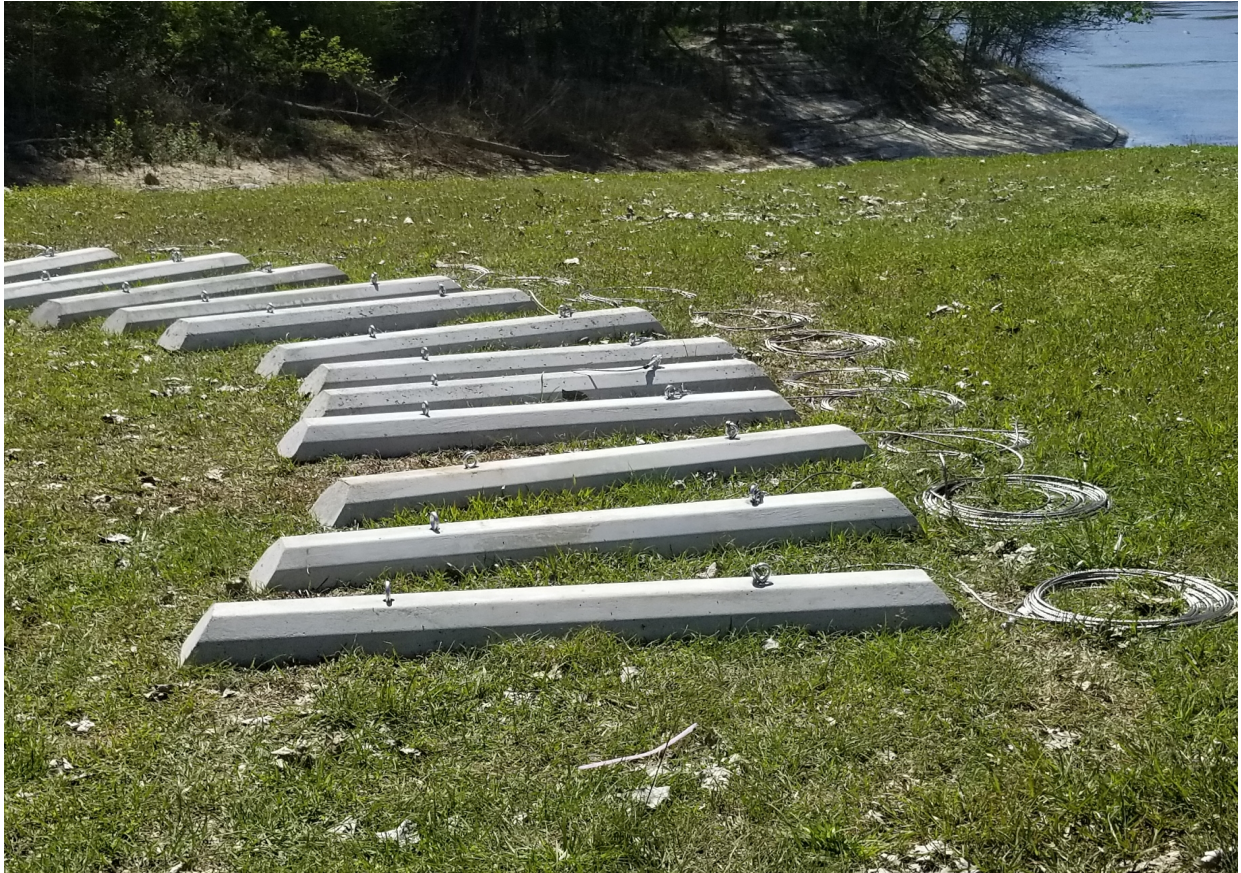
Figure A-3: Concrete parking stops with eyebolts and 100 feet of cable attached.
