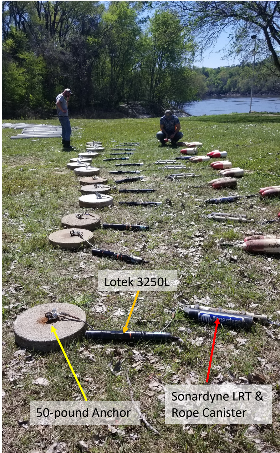
Figure A-4: The 50-pound anchor is attached to the Lotek 3250L and Sonardyne LRT with rope canister via a 6 to 10ft cable.
