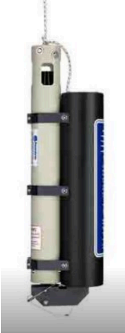
Figure A-2: Lightweight Release Transponder with rope canister used in the tailrace array to release the buoys.
