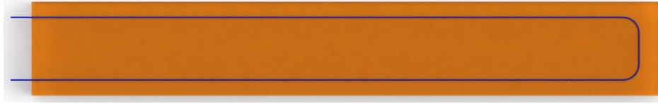
Figure 4.1: Bimorph SMA actuator with TPU substrate and RTV silicone coating (CAD Model - Top View)
