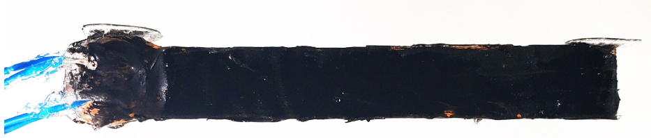
Figure 4.3: Bimorph SMA actuator with TPU substrate and RTV silicone coating and motion tracking markers (Top View)
