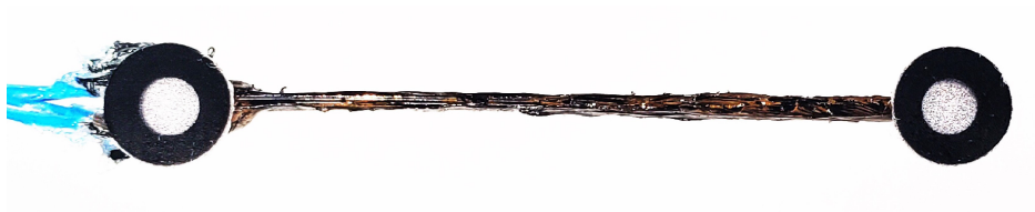
Figure 4.4: Bimorph SMA actuator with TPU substrate and RTV silicone coating and motion tracking markers (Side View)
