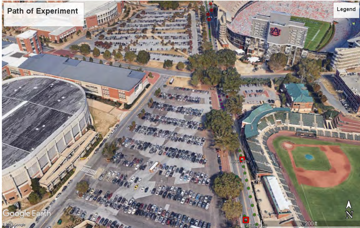
Figure 3.7: Portion of experiment when DRTK solution was lost under foliage and obstruction by Jordan-Hare stadium.
