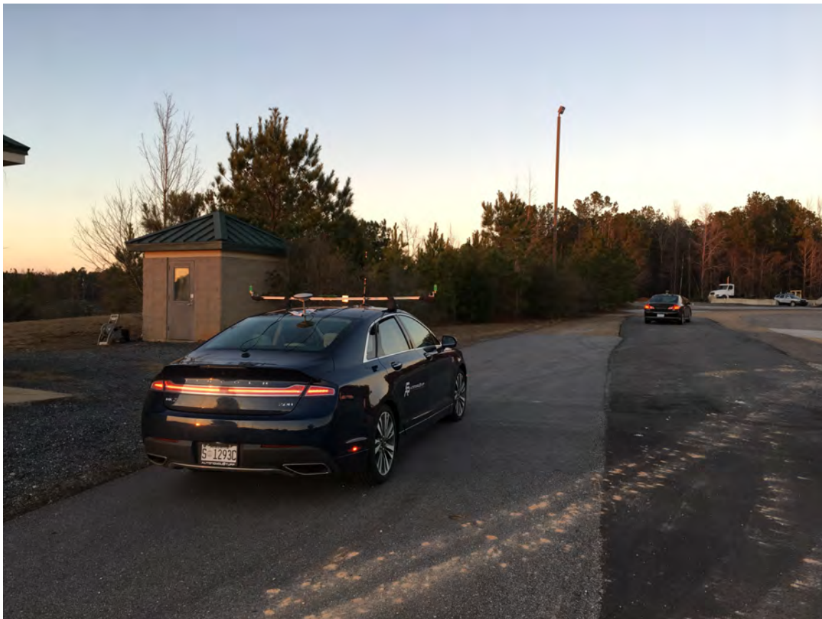
Figure 5.4: Lincoln Mkz and Infiniti G35 in the leader-follower configuration used for data collection.
