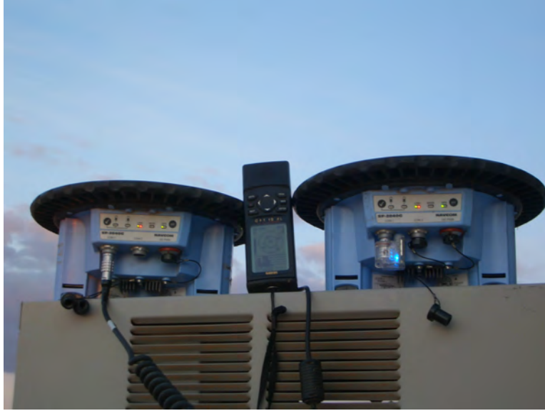
Figure 1.4: Two Navcom SF-2040G StarFire GPS receivers, along with a Garmin 12XL handheld. The Navcom on the right is using a Bluetooth serial adaptor. Source: [1]
