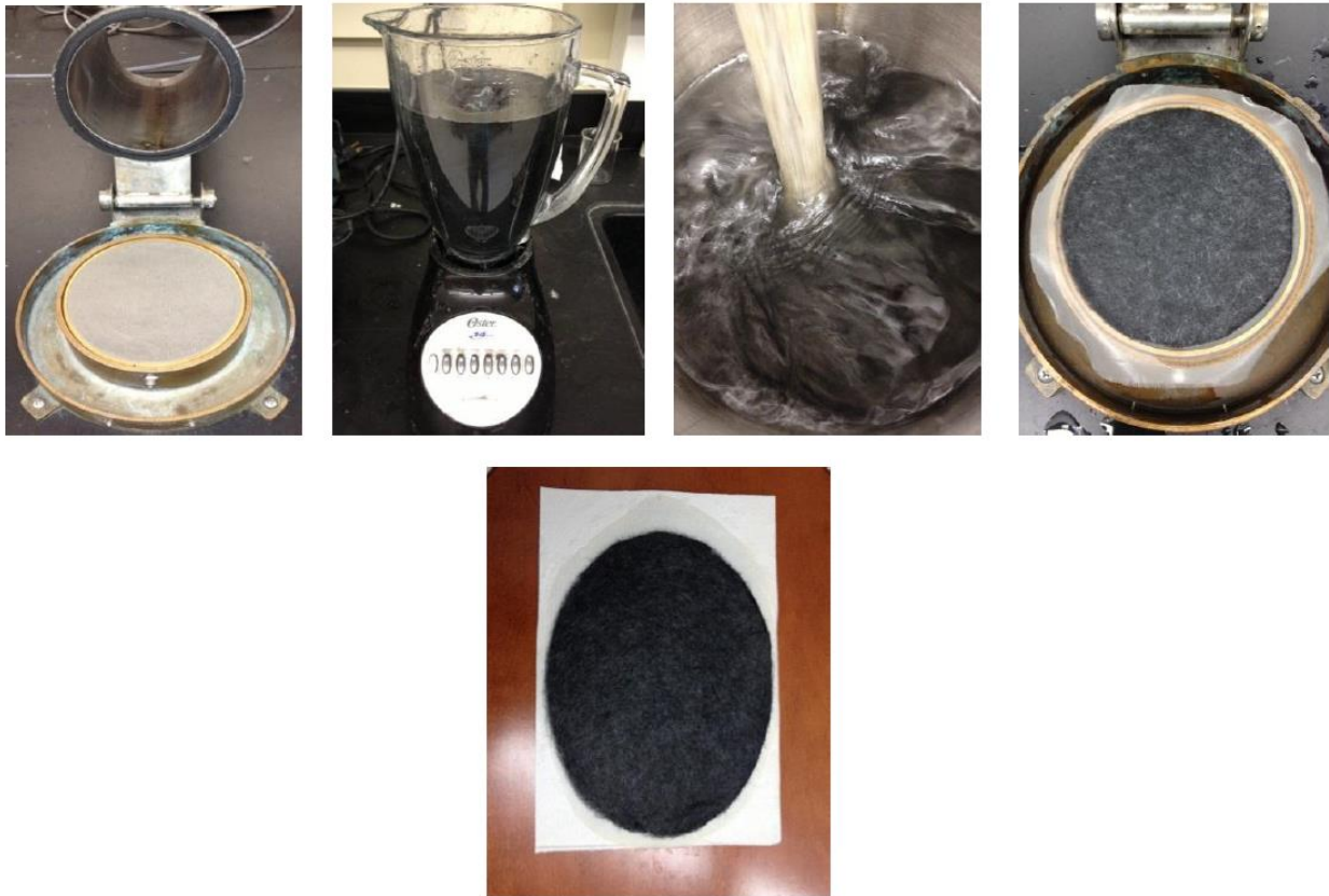
Figure 20. Wet-laid process of synthesizing AU Nano-floc filter media 1
