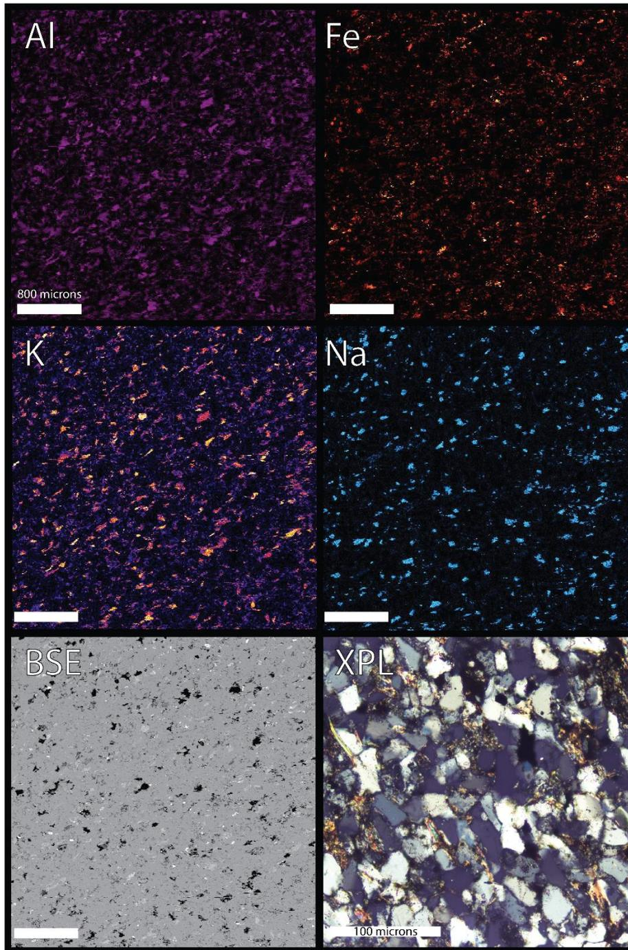
*Figure 19: High resolution compositional map of Pennsylvanian Atoka sandstone (OK12-1). Compositional maps analyzed for Al -Aluminum, Fe – Iron, K – Potassium, Na – Sodium, and BSE – Back Scattered Electron images. XPL – is a representative thin section image in cross polars showing monocrystalline quartz and metamorphic lithic fragments.*
