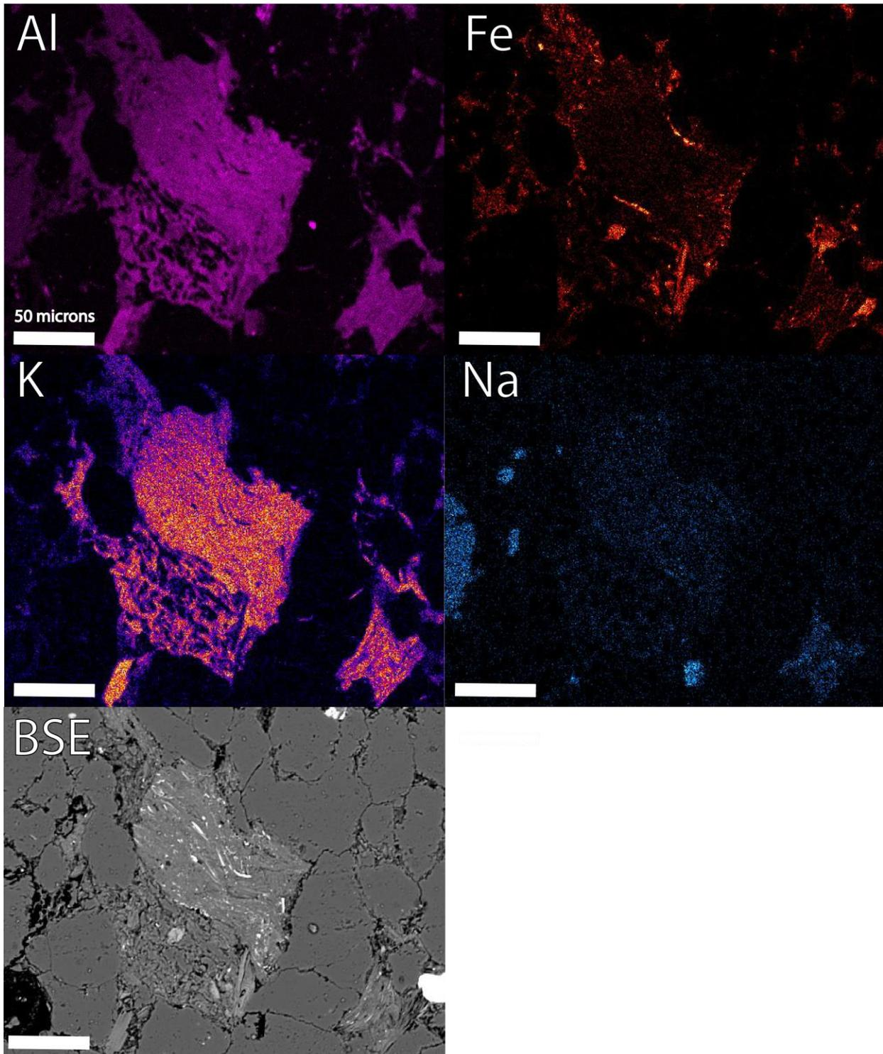
Figure 21: High resolution compositional map of a lithic fragment within the Pennsylvanian Atoka OK12-1 sample. Compositional maps analyzed for Al -Aluminum, Fe – Iron, K – Potassium, Na – Sodium, and BSE – Back Scattered Electron images. Thin crystals with high brightness in the BSE image and high Fe, are interpreted to be ilmenite.
