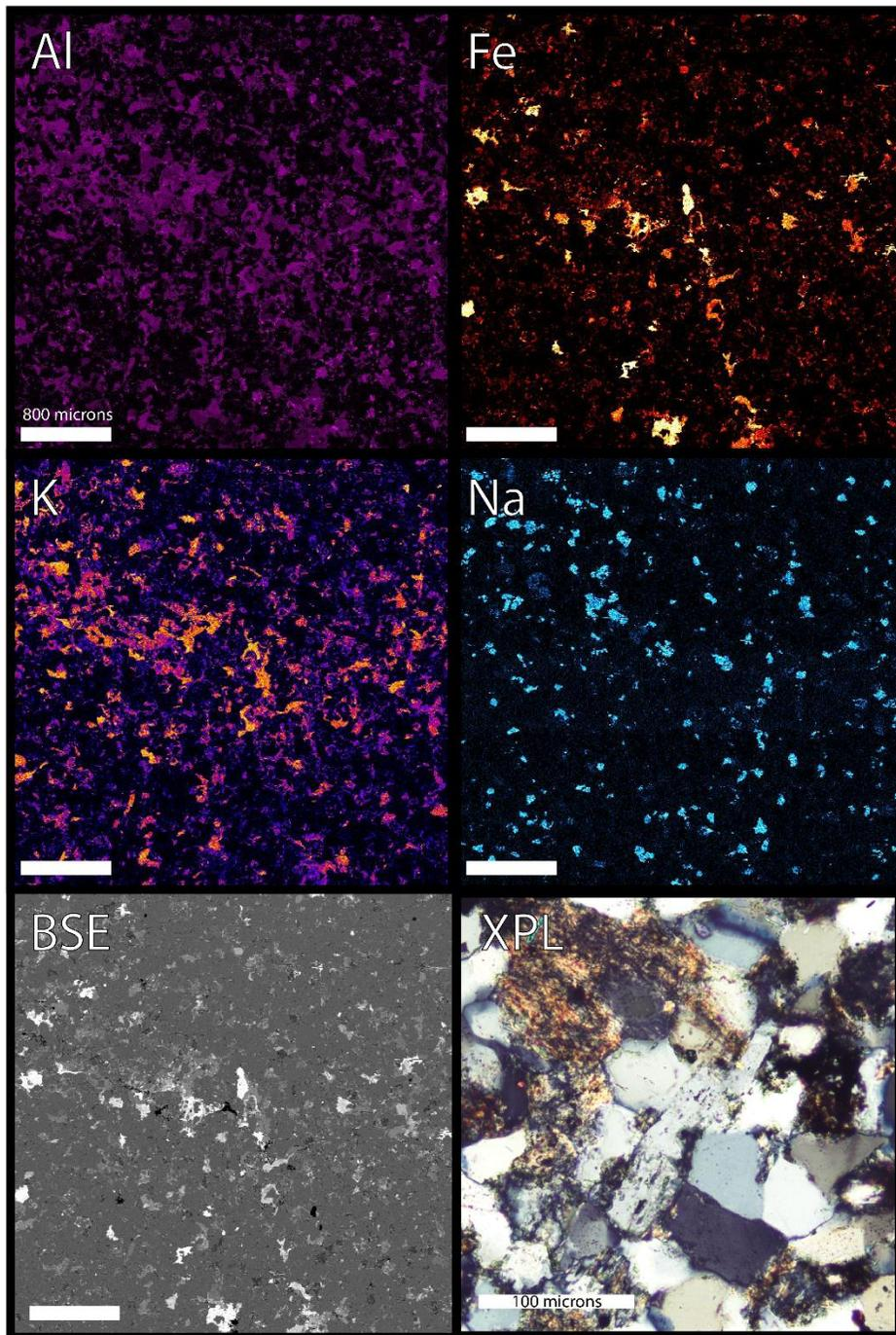
*Figure 20: High resolution compositional map of Pennsylvanian Atoka sandstone (OK12-4). Compositional maps analyzed for Al -Aluminum, Fe – Iron, K – Potassium, Na – Sodium, and BSE – Back Scattered Electron images. XPL – is a representative thin section image in cross polars showing monocrystalline quartz and metamorphic lithic fragments.*
