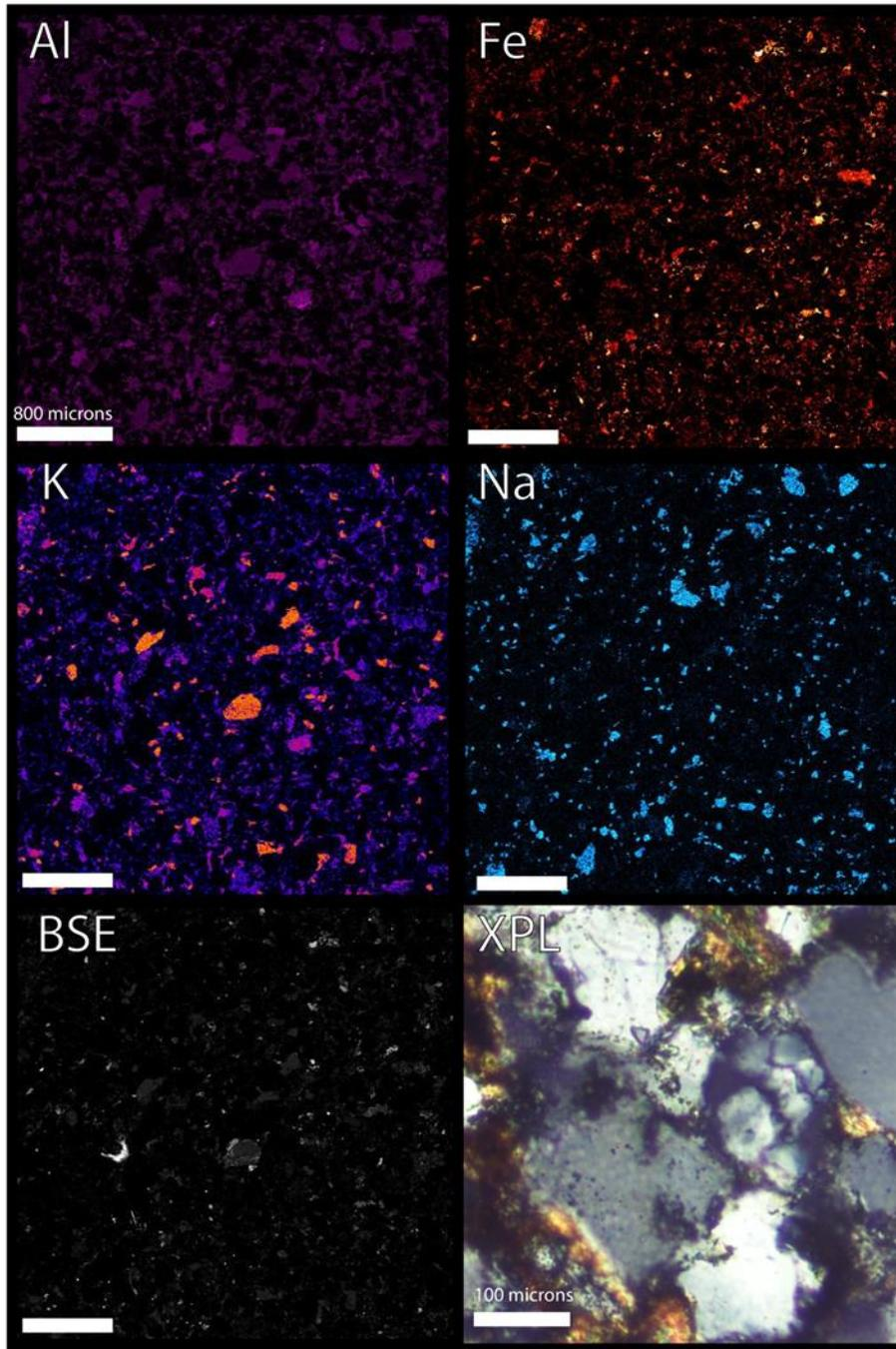
*Figure 18: High resolution compositional map of Pennsylvanian Atoka sandstone (OK12-32). Compositional maps analyzed for Al -Aluminum, Fe – Iron, K – Potassium, Na – Sodium, and BSE – Back Scattered Electron images. XPL – is a representative thin section image in cross polars showing monocrystalline quartz and metamorphic lithic fragments.*
