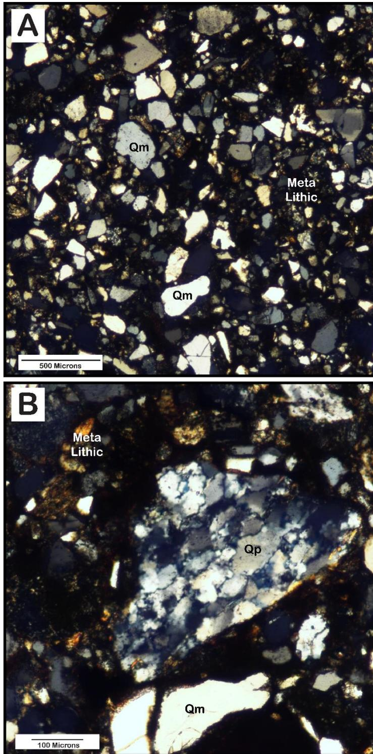
*Figure 13: Photomicrograph in cross polarized illumination of Mississippian Stanley sample OK12-31 showing in the top image (A) an abundance of matrix/pseudomatrix along with monocrystalline quartz (Qm) and lithic components. The bottom image (B) shows polycrystalline quartz (Qp), matrix, and lithic components.*
