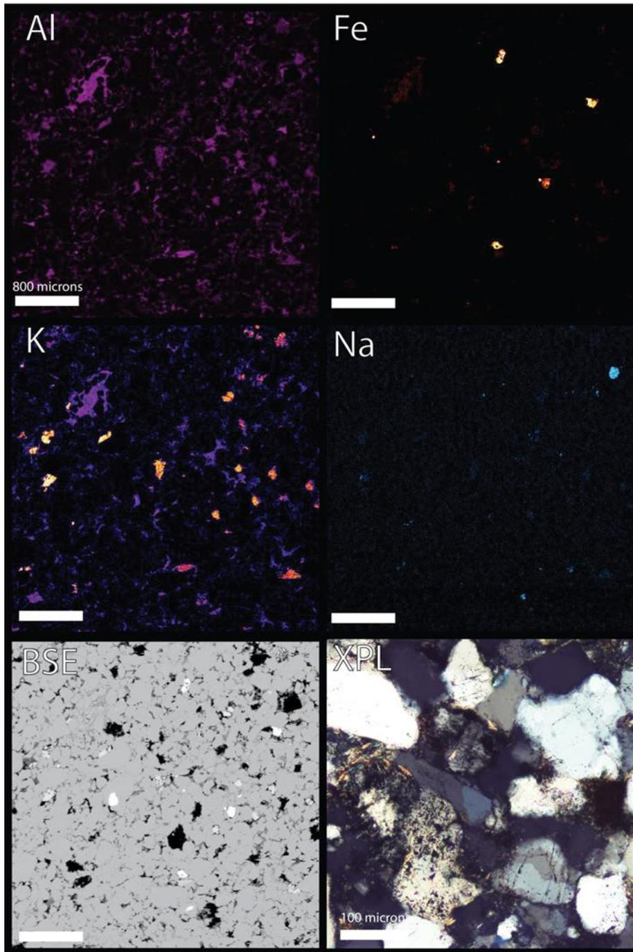
Figure 14: High resolution compositional map of Pennsylvanian Atoka sandstone (OK12-23). Compositional maps analyzed for Al -Aluminum, Fe – Iron, K – Potassium, Na – Sodium, and BSE – Back Scattered Electron images. XPL – is a representative thin section image in cross polars showing monocrystalline quartz and metamorphic lithic fragments.
