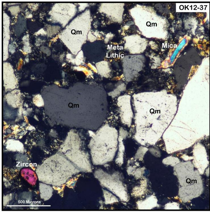
Figure 14: Photomicrograph of Pennsylvanian Jackfork samples OK12-50 and OK12-37. The samples show quartz dominated sandstones with minor metamorphic lithic components and presence of mica and zircons.
