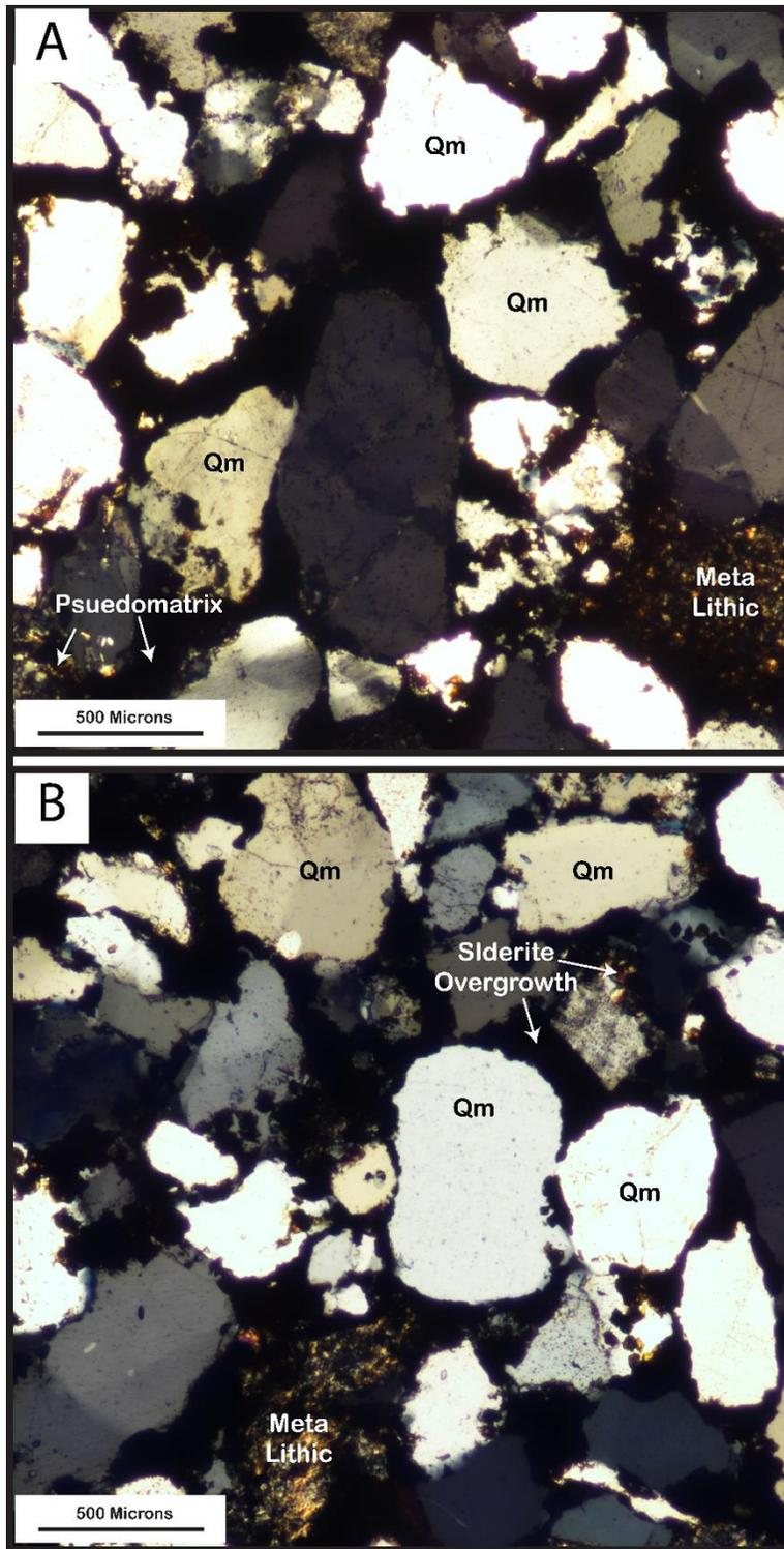
*Figure 15: Photomicrograph of Pennsylvanian Atoka Formation sample OK12-45. The photomicrograph shows jagged grain boundaries with clay and siderite overgrowth and a significant pseudomatrix component.*
