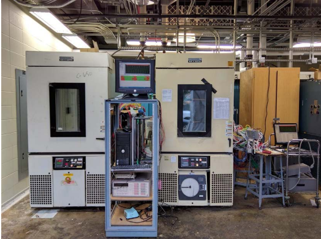
Figure 5.16 Thermal cycling chambers
