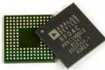
Figure 1.9 Top and bottom view of BGA package
