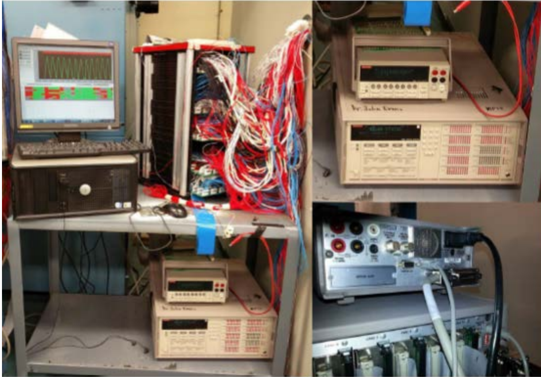
Figure 5.17 Full monitoring system (left) Keithley switching system and Digital Multimeter (DMM) from the front (right, top) and back (right, bottom). The DMM is sitting on top of the switching system [1]
