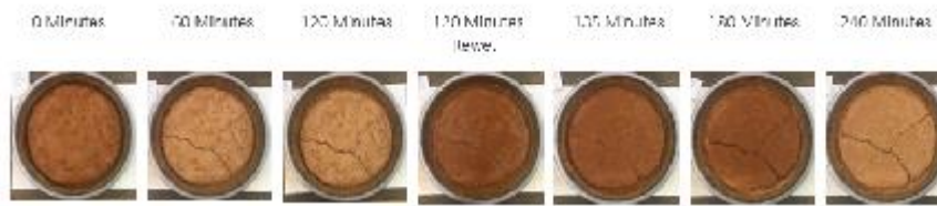
Figure 4. Desiccation crack test results for accelerated test for base soil.
