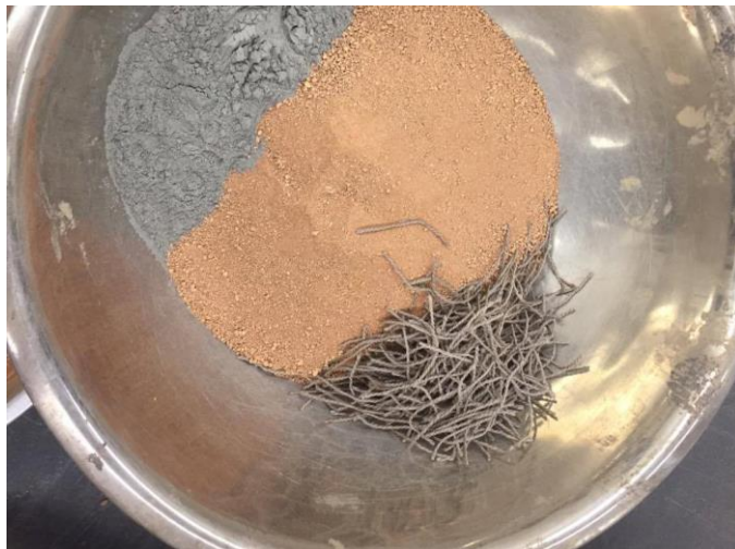
Figure 3.5 Dry Piedmont soil with fly ash and carpet fibers.
