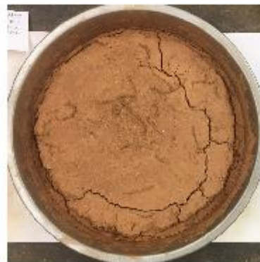
Figure 5. Accelerated test final crack distribution for fiber-aided soil.
