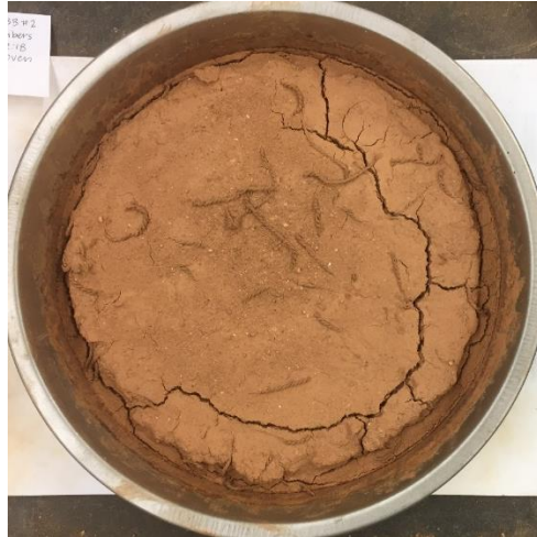
Figure 5.3 Accelerated test final crack distribution for fiber-aided soil
