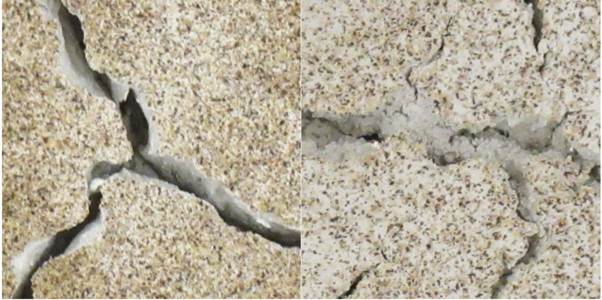
Figure 5.13 Comparison of cracks in kaolinite soil in: a) untreated samples b) xanthan gum aided samples
