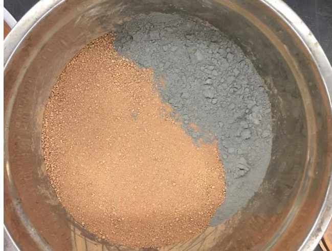
Figure 3.3 Dry Piedmont soil with fly ash.
