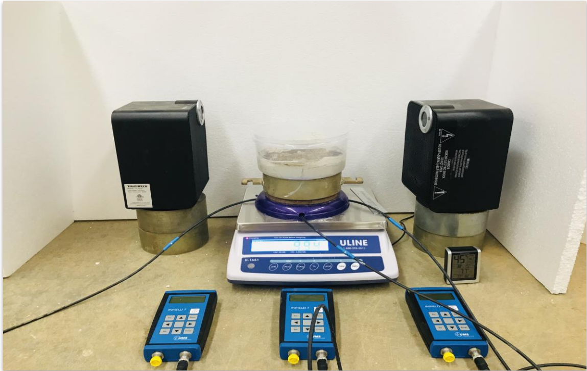
Figure 3.9 Setup for desiccation test of kaolinite clay.
