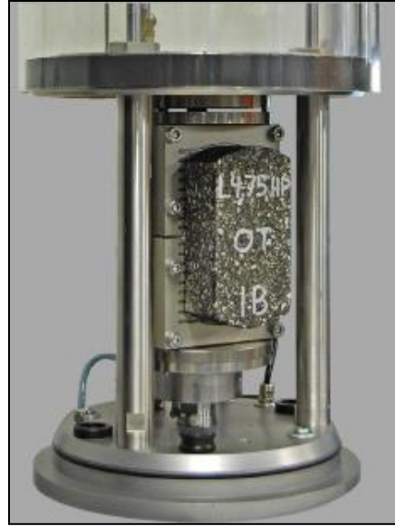
Figure 3. 10 TX-OT Specimen Setup
