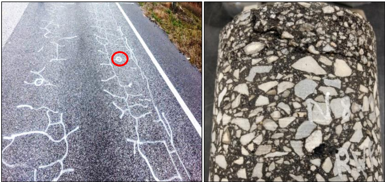
Figure 1. 1 Typical TDC and a Corresponding Field Core
