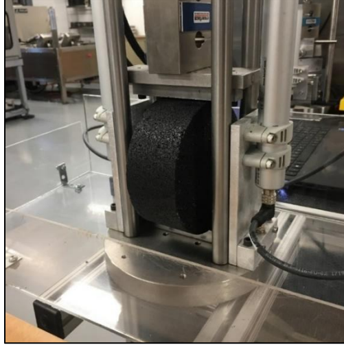
Figure 3. 17 IDEAL-CT Test Setup
