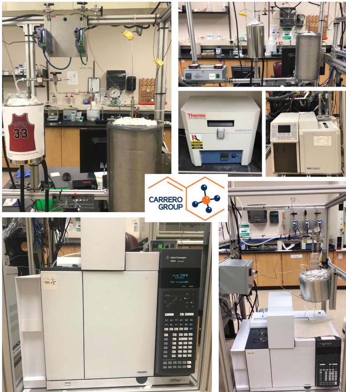
Actual reactor setup, showing mass flow controllers, temperature controller, furnace, chiller, transfer line, and GC.
