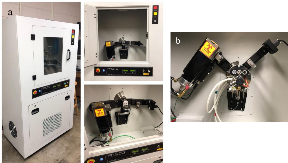
Figure 26. (a) XRD diffractometer to analyze the crystal structure of the catalyst, (b) equipped with an XRK-900 (Anton par) in-situ cell.
