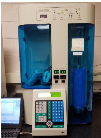
Figure 25. NOVA nitrogen physisorption equipment for the determination of surface area.
