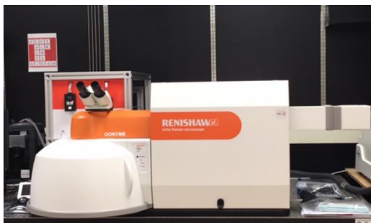
Figure 27. In via Raman spectrometer with Qontor technology for the analysis of vibrational modes present in the material.
