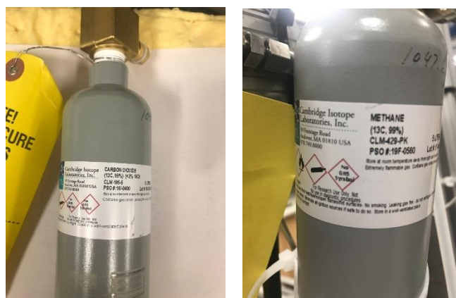
Figure 24. Isotopic labelled gases (a) ^{13}\text{CO}_2 and (b) ^{13}\text{CH}_4 for mechanistic steady-state DRM reaction studies from Cambridge Laboratories Inc, California.
