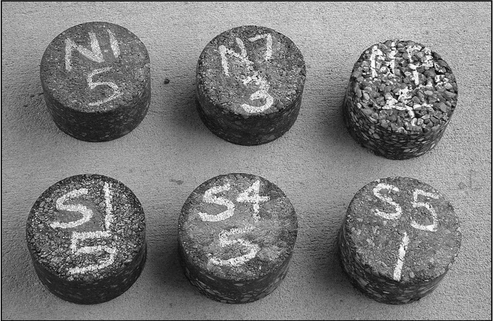
Figure 6.3. The 3-inch thick hard surface dense track pavement samples
