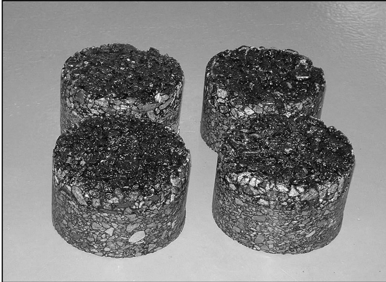
Figure 6.13. OGFC graded coarse 1.5-inch thick 6-inch diameter porous cores
