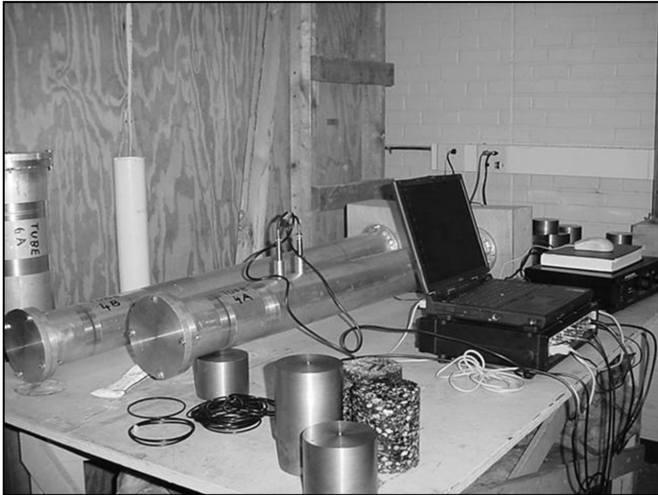
Figure 6.2. Experimental setup, 4-inch impedance tubes, asphalt cores, “O” rings and metal back plates. Shown as well is the Brüel & Kjaer Pulse System. The 6-Inch tube can also be seen in the back ground.
