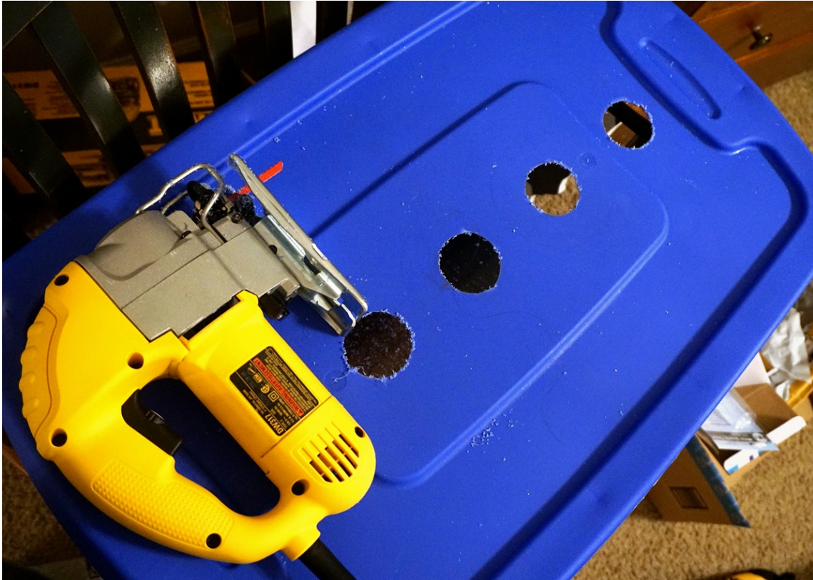
Figure 25: Construction of Growth Chamber and Nutrient Reservoir.
