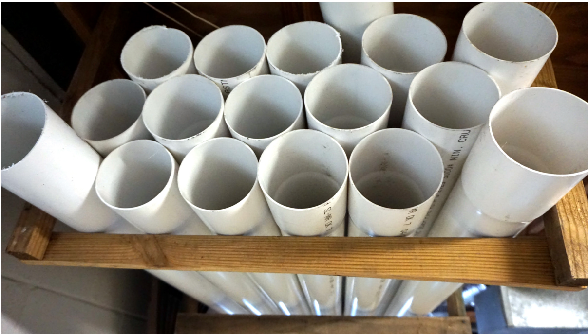
Figure 49: 4" PVC Pipe Used for HPA Vertical Tower Prototype.
