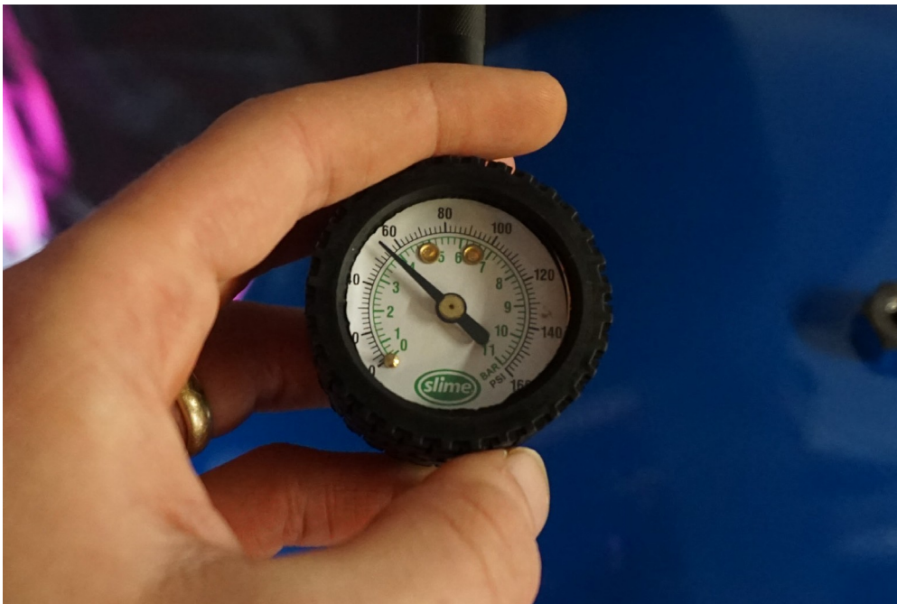
Figure 41: Pressure Reading Displaying Need for Additional Pressure.
