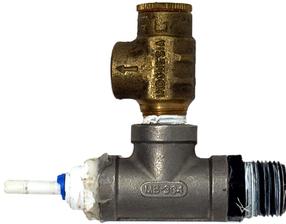
Figure 20: Relief Valve Setup for HPA System.
