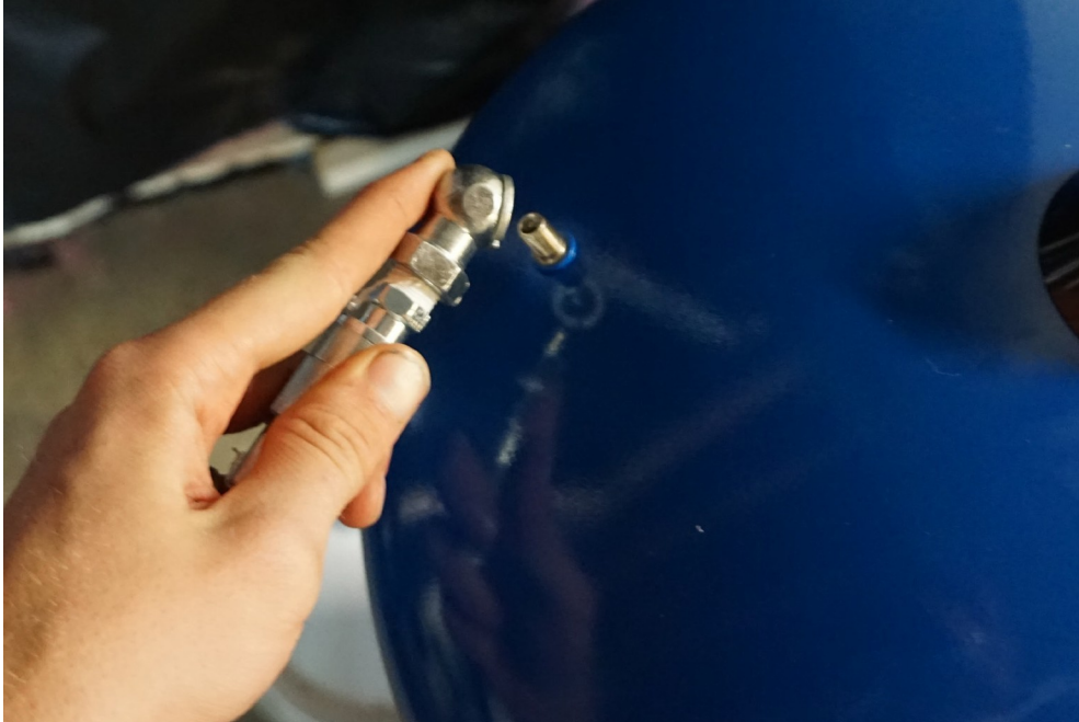
Figure 40: Pressure Added to Accumulator Tank.
