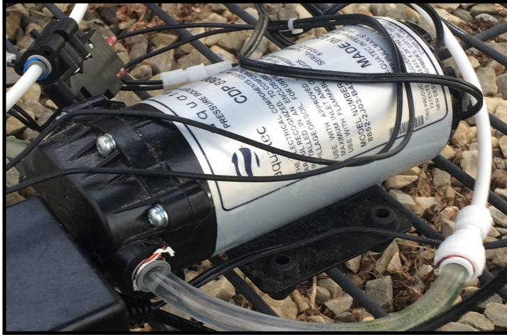
Figure 37: Booster Pump Used in HPA Prototype.
