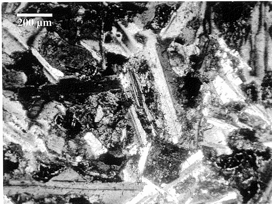
Figure 6: Thin section of the dolerite sample from the study area under crossed polars illustrating subophitic texture.
