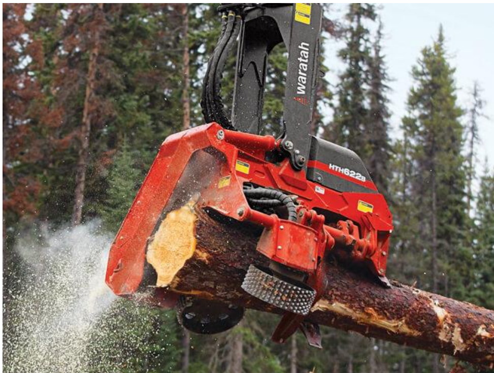
Figure 10. Waratah HTH622B that depicts the location of trimming saw and feed wheels (Waratah n. d.)
