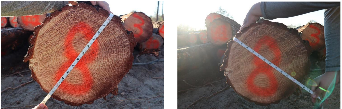
Figure 12. Two different diameter readings from the same log
