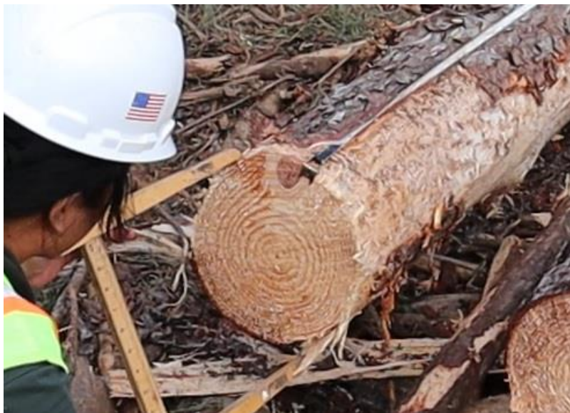
Figure 15. Knots on the section of a log where post measurement was taken
