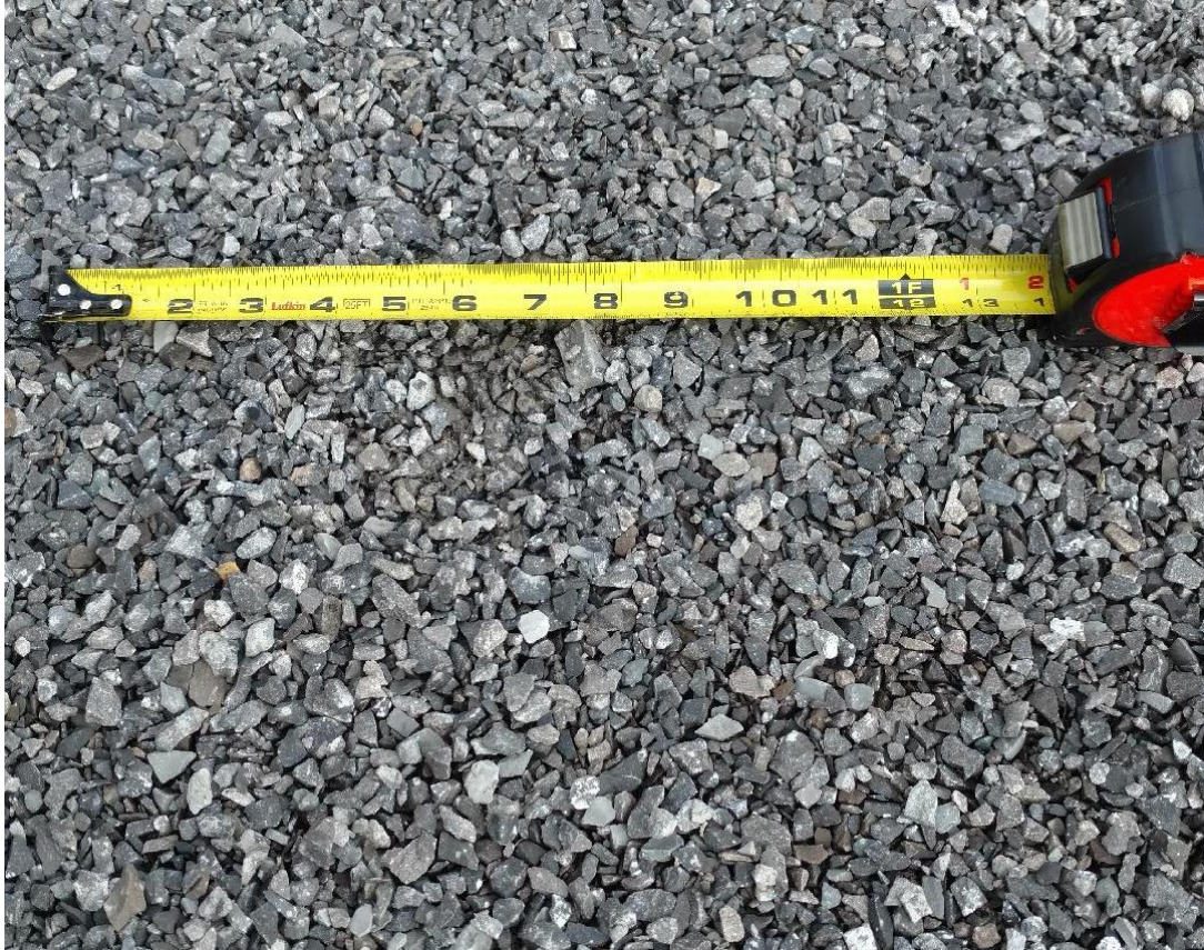
Figure 28. AASHTO No. 89 aggregate.
