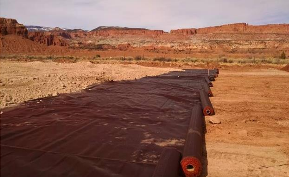
Figure 7. Woven geosynthetic reinforcement material. Geosynthetics are generally stored in rolls (Tencate Geosynthetics 2020).
