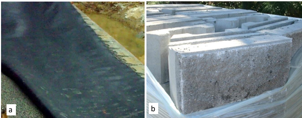
Figure 30. (a) Selected woven geosynthetic; (b) segmental retaining wall masonry units (from Hogan 2018).
