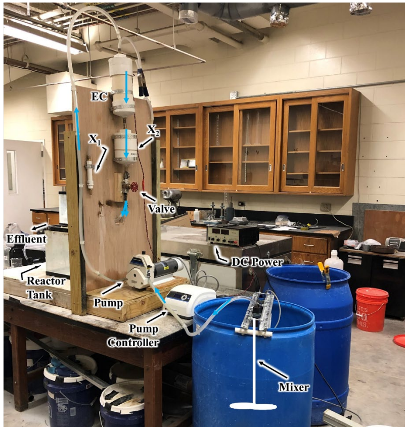
Figure 5.3 EC+LS Experimental Setup.
