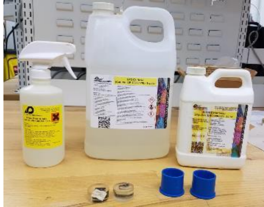
Figure 5.15: Cleaner, Resin, Hardener (rare line from left to right), Samples and Molds (front line)
