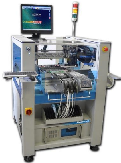
Figure 2.13: Example of Pick-and-Place Machine
