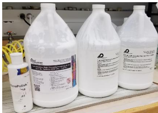
Figure 5.17: Polishing Alumina Suspension of Various Sizes (First Three from Right) and Colloidal Silica Solution
