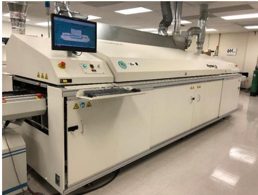
Figure 4.3 : 8-zone Pyramax 100N Reflow Oven
