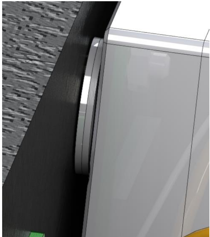
Figure 29: Belleville Washer Between Battery Pack and +Y Face
