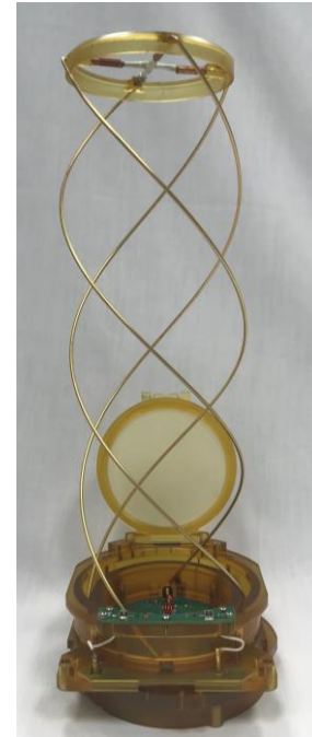
Figure 91: HCT Shape Memory Alloy Deployable Travelling-Wave Antenna, Used with Permission [132]
