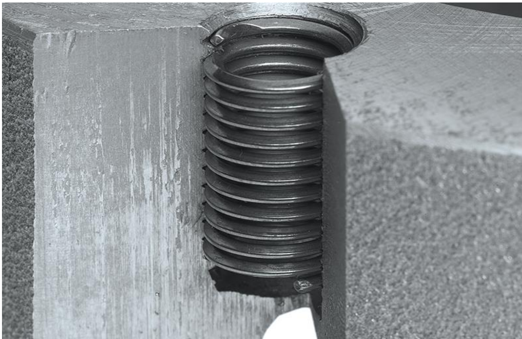
Figure 28: Thread Locking Helicoil from Boellhoff, Used with Permission [45]
