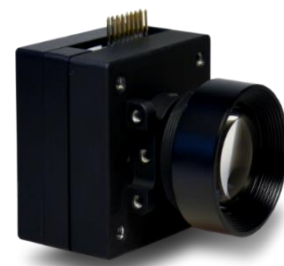
Figure 97: Hyperion ST200 Shown Without Baffle. Baffles are commonly 30 or 45 degrees, used with permission [186]
