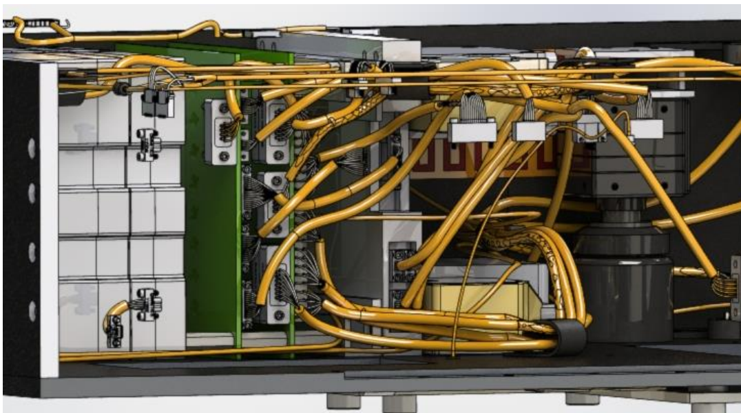
Figure 21: -X View, Interior Cable Harnessing Design
