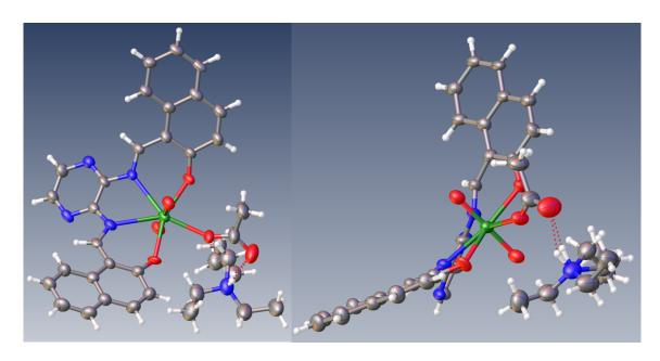
Figure 4.31. Naphthylpyrasal- UO<sub>2</sub> crystal structure grown from DCM/Hexane. Atoms shown are labeled: H in white, O in red, N in blue, C in grey, U in green.
