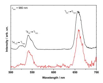
Figure 3.23. Two-photon UC emission spectra of (a) [(Yb0.78Er0.22)2(L-CN)3(H2O)] (black upper trace) and [Er2(L-CN)3(H2O)] (red bottom trace) in the solid state.  $\lambda$  exc = 980 nm, P = 2.5 W.
