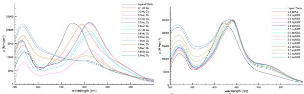
Figure 2.12. Methoxysalimidizine (L3) titrations with  $Cu^{2+}$  acetate (left) and  $UO_2^{2+}$  acetate (right).
