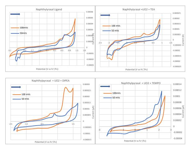
Figure 4.34. Cyclicvoltammagrams of Naphthylpyrasal ligand and alternate reaction (TEA, DIPEA, TEMPO) conditions in DCM 400  $\mu$ M with TBAPF<sub>6</sub>
