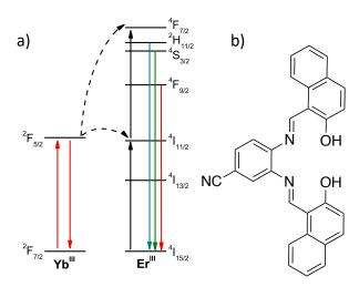
Figure 3.18. a) Energy level diagram illustrating the up-conversion process through ESA (two black up-arrows on  $E^{III}$ ) and ETU (dashed arrows, red up-arrow on  $Y^{III}$  followed by top black up-arrow on  $E^{III}$ ). b) Structure of  $H_3L$ -CN
