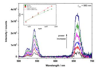
Figure 3.22. Two-photon UC emission spectra of  $[(Y_{0.76}Yb_{0.16}Er_{0.08})_2(L-CN)_3(H_2O)]$  in the solid state using variable laser power. Inset shows plot of the log of the emission intensity I at 543 nm (green dots) or 655.5 nm (red dots) as a function of the log of the laser power P.  $\lambda_{exc} = 980$  nm, P = 0.873 - 2.500 W.
