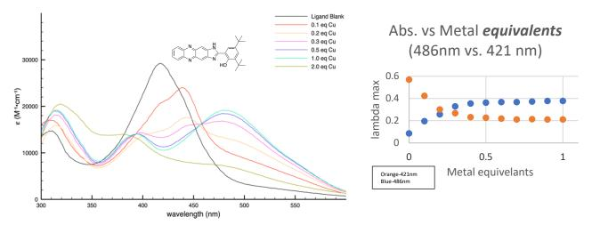
Figure 2.10. Ditertbutyl-salimidizine titration with  $Cu^{2+}$  acetate (Left);  $\lambda$  max vs. metal equivalents @ 486nm and 421nm.(right)
