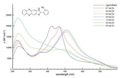
Figure 2.9. Salimidizine (L1) titration with Cu<sup>2+</sup> acetate
