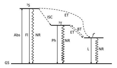
Figure 1.6.Modified Jablonski Diagram demonstrating the antenna effect for lanthanide complexe. 68
