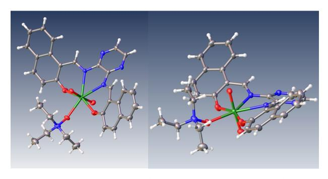
Figure 4.30. Single crystal structural representation of the Naphthylpyrasal-  $UO_2$  crystal structure as grown from 1:1 1,4-dioxane/pentane top view(Left) and side view (Right). Atoms shown are labeled: H in white, O in red, N in blue, C in grey, U in green. Solvent molecules within the unit cell are removed for clarity.
