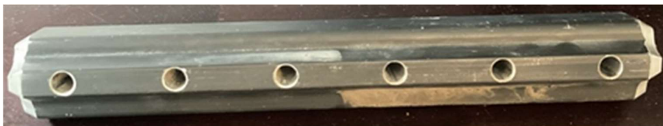
Figure 3.1-7. Side view of splice member
