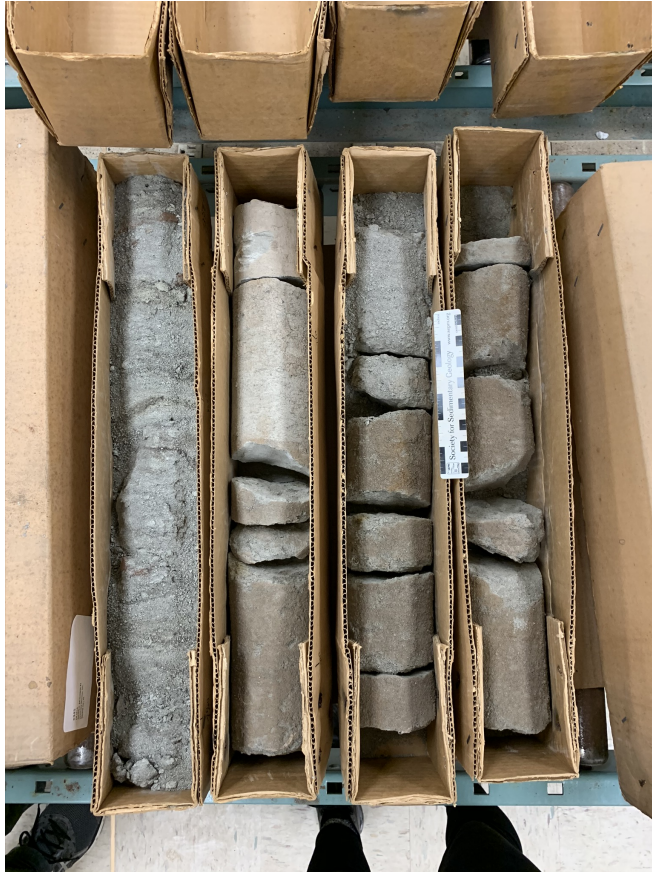
Figure 1.18: Section of the Julian F. McGowin #1 drill core. This section is part of the Pilot sands of the lower Tuscaloosa. This section of the core contained large amount of muscovite. Depth ranges from 2242 m, and 2350 m – 2351 m (7358 ft and 7711-7716 ft).
