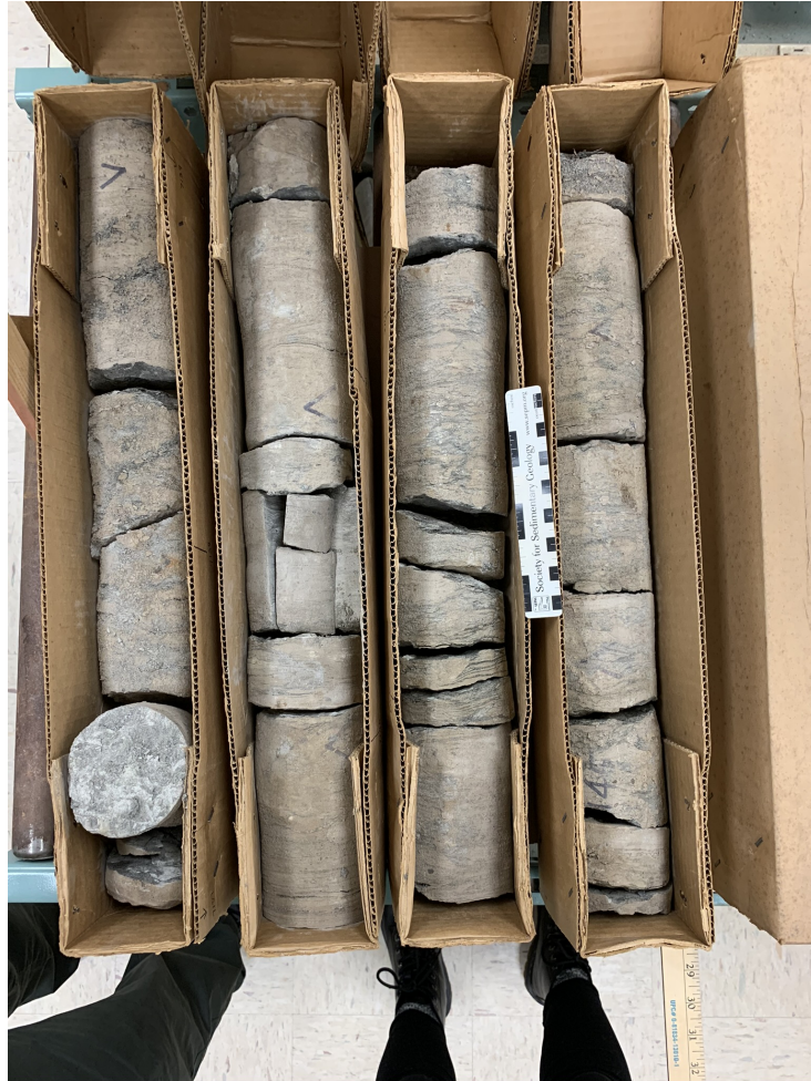
Figure 1.21: Section of the Julian F. McGowin #1 drill core. Glauconite was not as abundant as the last section of the core. This section is also the top of the drill core. Depth ranges from 2175 m – 2177 m (7137 ft – 7145 ft).
