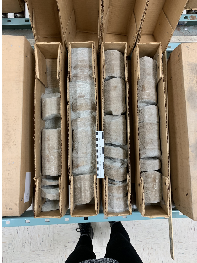
Figure 1.4: Section of the Julian F. McGowin #1 drill core. This section is part of the Massive sands of the lower Tuscaloosa. Depth ranges from 2562 m – 2563 m (8408 ft – 8411 ft).
