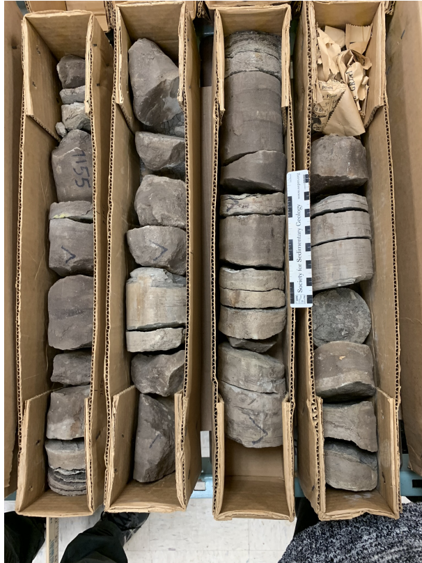
Figure 1.19: Section of the Julian F. McGowin #1 drill core. This section is part of the of the sandstones that make part of the upper Tuscaloosa. Glauconite was not as abundant as the last section of the core. Depth ranges from 2180 m – 2183 m (7154 ft – 7163 ft).
