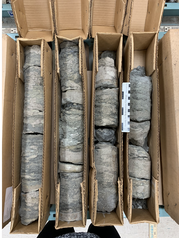
Figure 1.12: Section of the Julian F. McGowin #1 drill core. This section is part of the Pilot sands of the lower Tuscaloosa. Glauconite was also very abundant in this section of the core. Depth ranges from 2366 m – 2368 m (7765 ft – 7772 ft).
