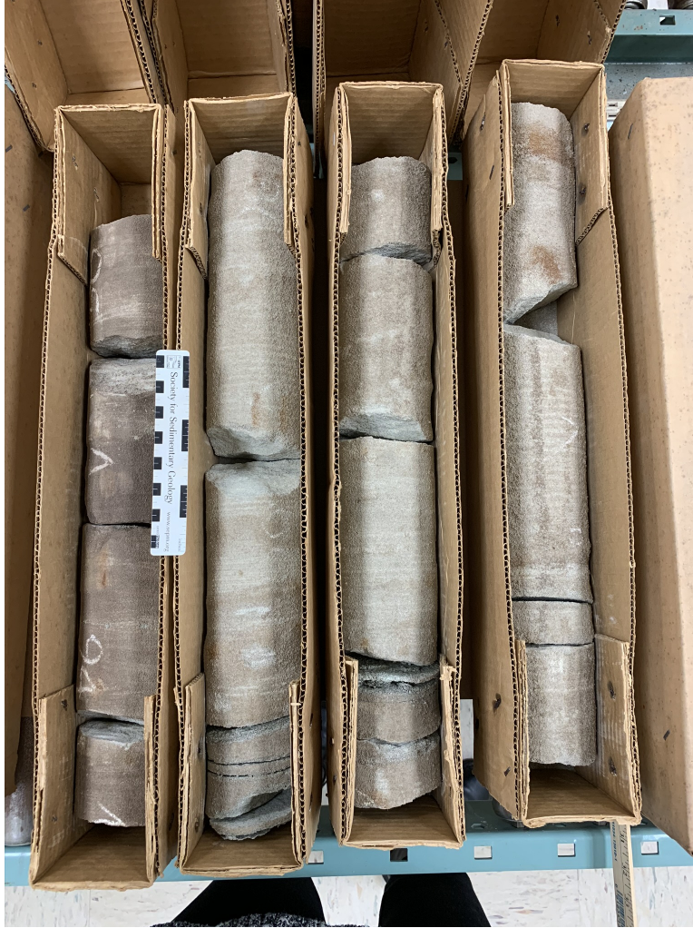
Figure 1.5: Section of the Julian F. McGowin #1 drill core. This section is part of the Massive sands of the lower Tuscaloosa. Depth ranges from 2560 m- 2562 m (8399 ft – 8408 ft).
