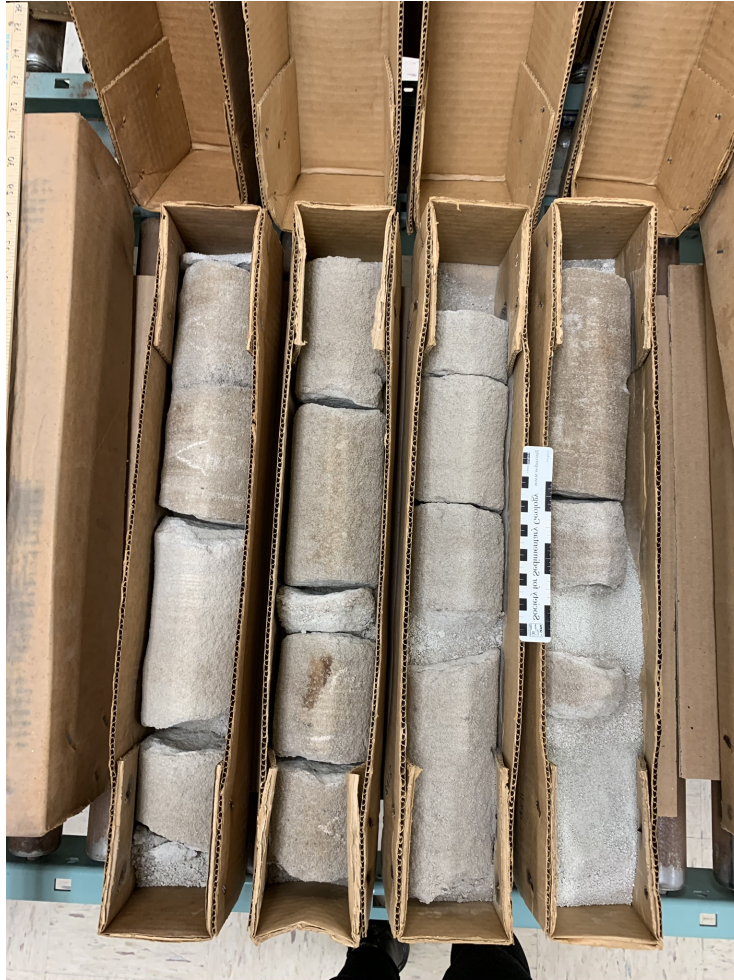
Figure 1.3: Section of the Julian F. McGowin #1 drill core. This section is part of the Massive sands of the lower Tuscaloosa. Depth ranges from 2563 m – 2568 m (8411 ft – 8427 ft).
