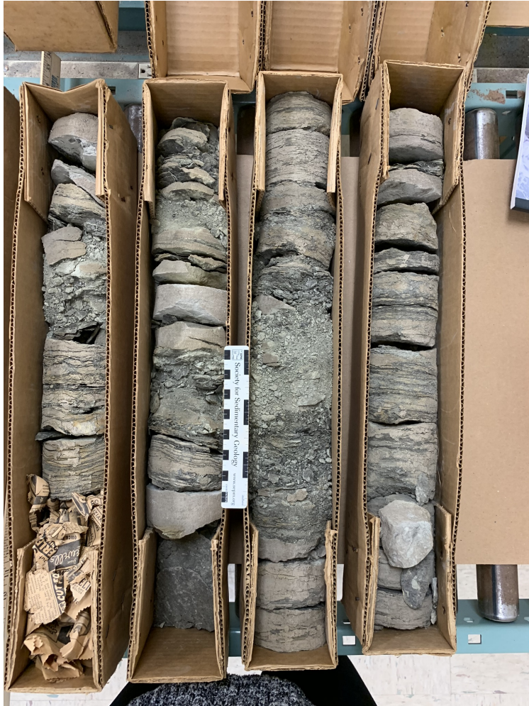
Figure 1.11: Section of the Julian F. McGowin #1 drill core. This section is part of the Pilots sands of the lower Tuscaloosa. The samples taken from this section were interbedded sandstones and shales. Glauconite was also very abundant in this section of the core 2382 m – 2385 m (7818 ft – 7826 ft).
