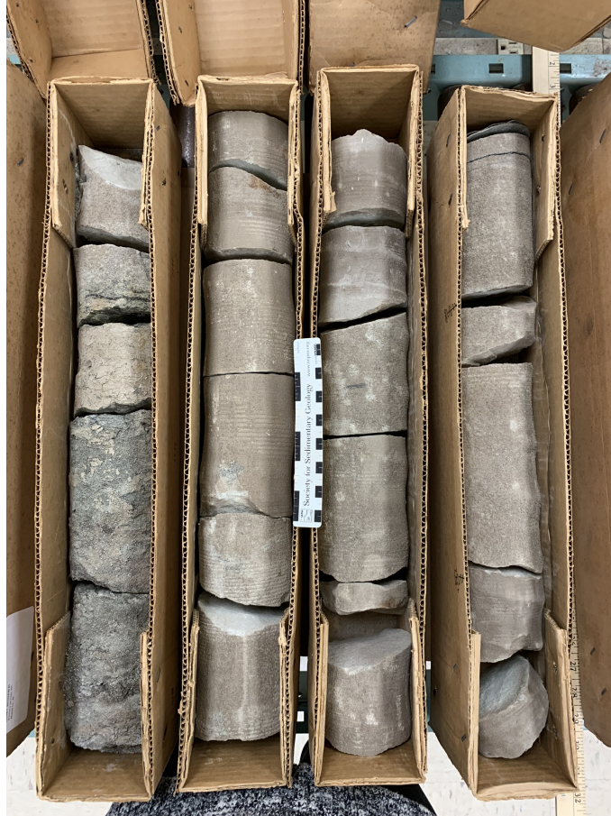
Figure 1.14: Section of the Julian F. McGowin #1 drill core. This section is part of the Pilot sands of the lower Tuscaloosa. Depth ranges from 2360 m – 2362 m (7743 ft – 7752 ft).
