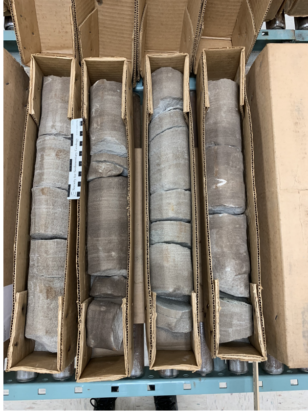
Figure 1.7: Section of the Julian F. McGowin #1 drill core. This section is part of the Pilot sands of the lower Tuscaloosa Potassium feldspar was abundant in these sections of the core. Depth ranges from 2399 m – 2551 m (7872 ft – 8370 ft).
