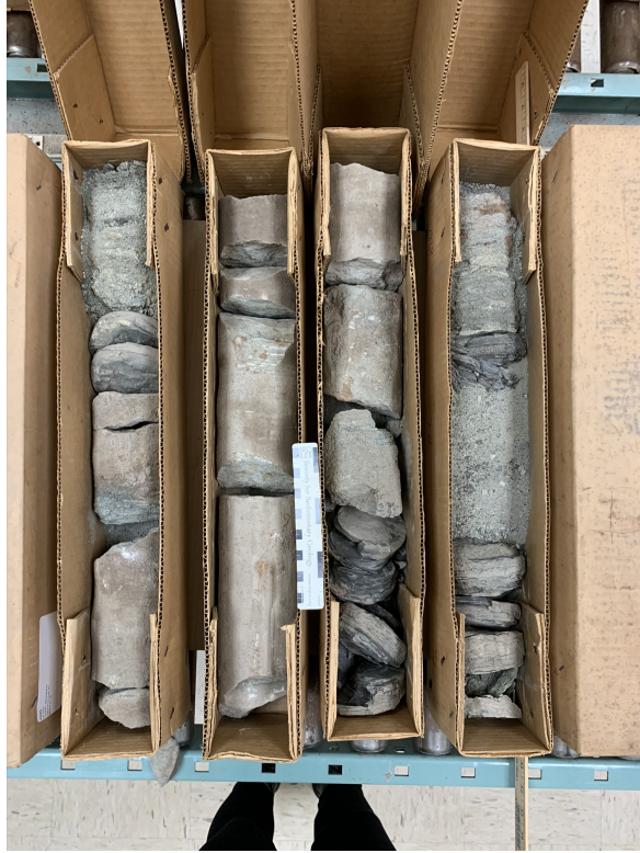
Figure 1.8: Section of the Julian F. McGowin #1 drill core. This section is part of the Pilot sands of the lower Tuscaloosa. There is clear distinction in lithology. These sandstones contained large amounts of glauconites. Depth ranges from 2394 m – 2399 m (7856 ft – 7872 ft).
