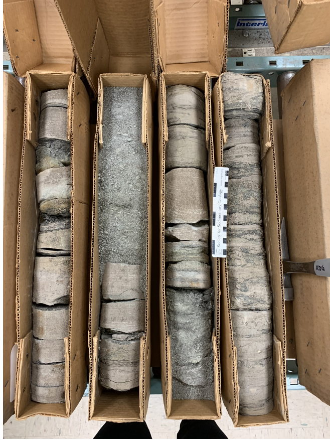
Figure 1.13: Section of the Julian F. McGowin #1 drill core. This section is part of the Pilot sands of the lower Tuscaloosa. Depth ranges from 2363 m – 2366 m (7753 ft – 7764 ft).
