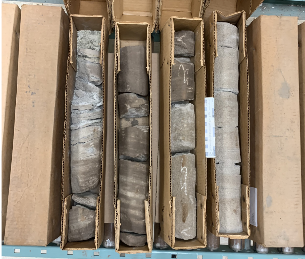
Figure 1.2: Section of the Julian F. McGowin #1 drill core. This section is part of the Massive sands of the lower Tuscaloosa. Depth ranges from 2566 m – 2568 m (8419 ft- 8427 ft).
