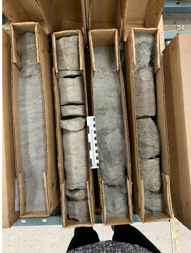
Figure 1.16: Section of the Julian F. McGowin #1 drill core. This section is part of the Pilot sands of the lower Tuscaloosa. Depth ranges from 2355 m – 2357 m (7727 ft – 7734 ft).
