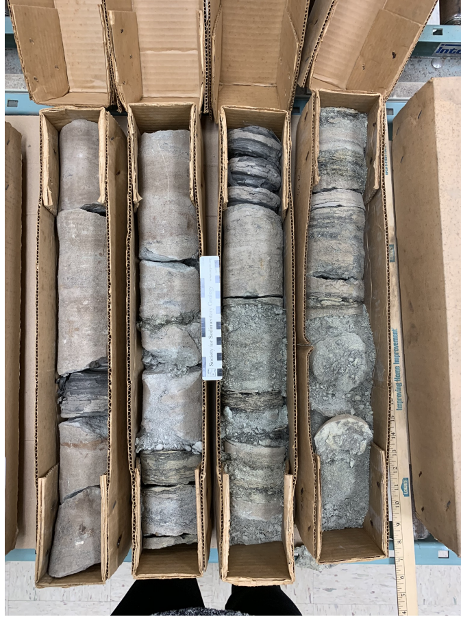
Figure 1.9: Section of the Julian F. McGowin #1 drill core. This section is part of the Pilot sands of the lower Tuscaloosa. The samples taken from this section were interbedded sandstones and shales. Glauconite was also very abundant in this section of the core. Depth ranges from 2389 m -2394 m (7840 ft – 7856 ft).
