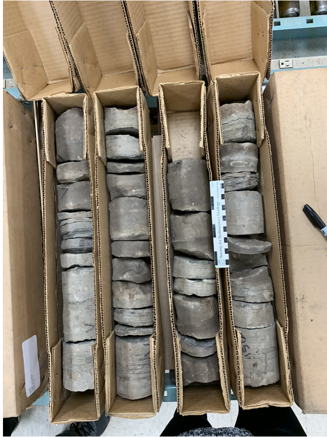
Figure 1.20: Section of the Julian F. McGowin #1 drill core. Glauconite was not as abundant as the last section of the core. Depth ranges from 2178 m – 2180 m (7148 ft – 7153 ft).
