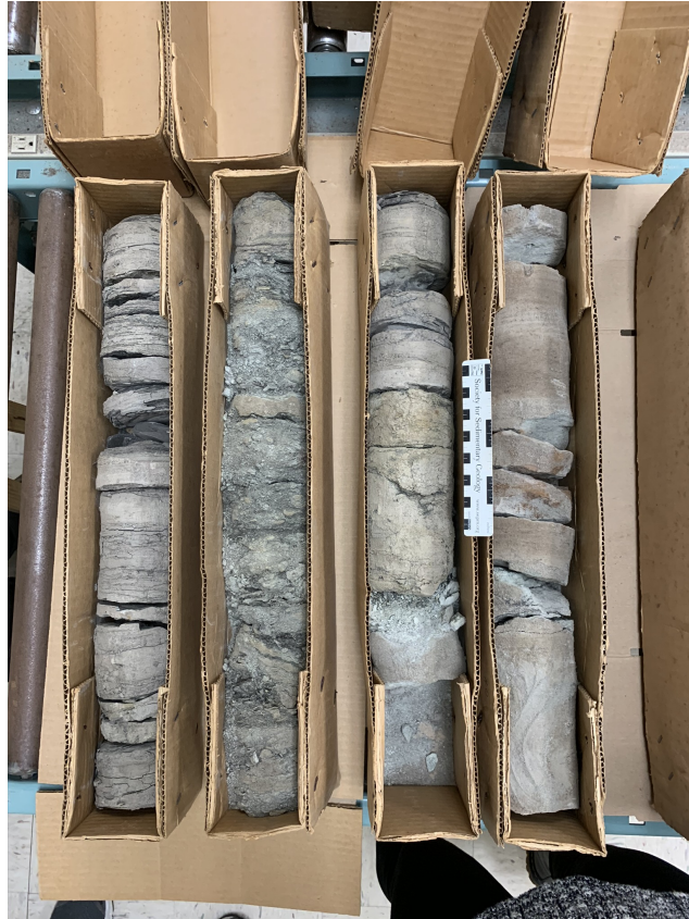
Figure 1.10: Section of the Julian F. McGowin #1 drill core. This section is part of the Pilot sands of the lower Tuscaloosa. The samples taken from this section were interbedded sandstones and shales. Glauconite was also very abundant in this section of the core. Depth ranges from 2385 m – 2389 m (7826 ft – 7840 ft).
