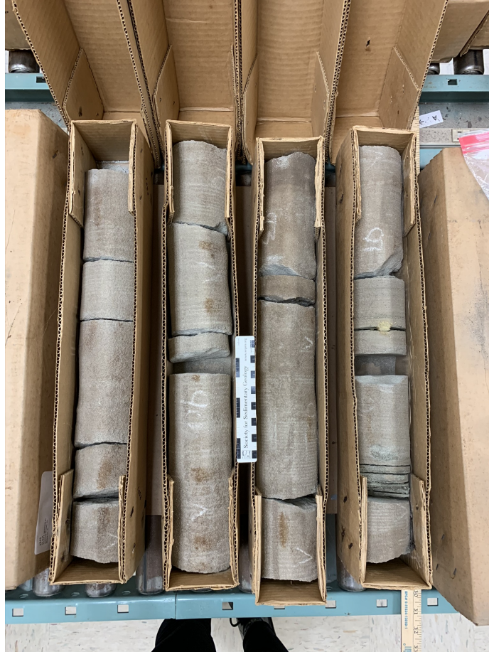
Figure 1.6: Section of the Julian F. McGowin #1 drill core. This section is part of the Massive sands of the lower Tuscaloosa. Depth ranges from 2556 m -2559 m (8387 ft – 8397 ft).
