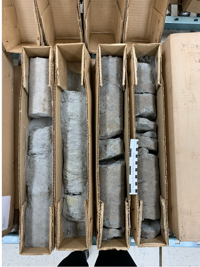
Figure 1.17: Section of the the Julian F. McGowin #1 drill core. This section is part of the Pilot sands of the lower Tuscaloosa. Depth ranges from 2352 m – 2354 m (7718 ft – 7726 ft).
