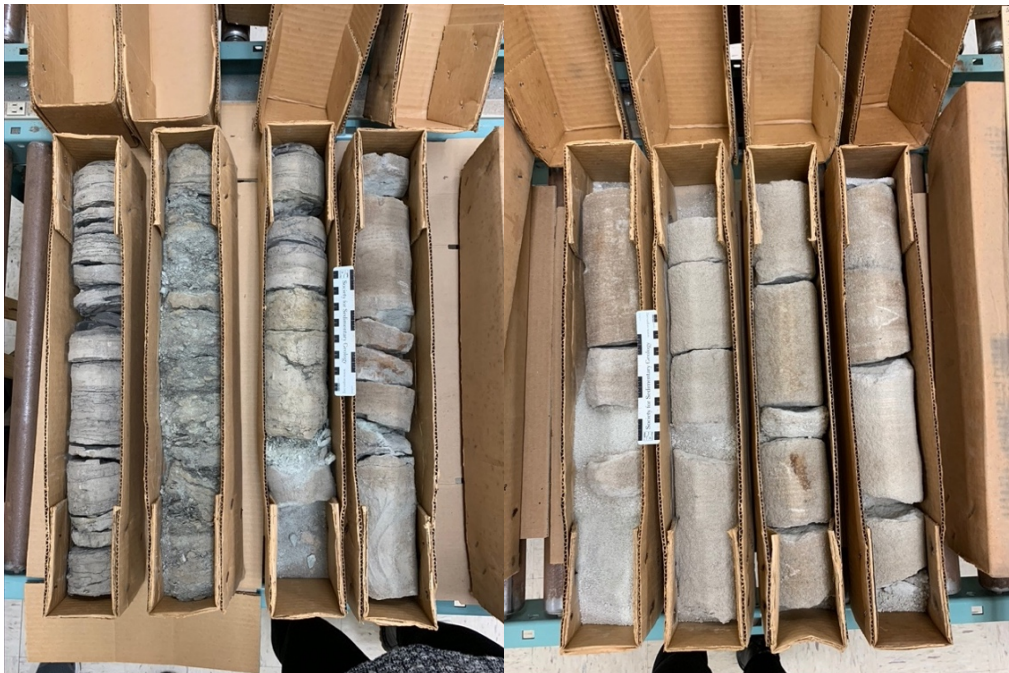
Figure 5: Sections from the Julian F. McGowin #1 (permit no. 1419) drill core. Drill core samples were obtained from the Geological Survey of Alabama. This drill core's overall depth ranges from 7137-8435 ft (2175 - 2571 m).
