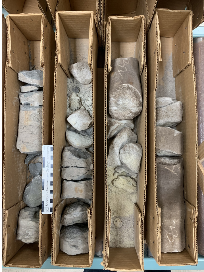
Figure 1.1: Section of the Julian F. McGowin #1 drill core. This section is part of the Massive sands of the lower Tuscaloosa. Depth ranges from 2568 m – 2570 m (8427 ft – 8435 ft).
