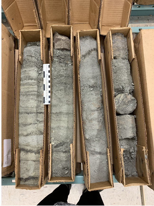
Figure 1.15: Section of the Julian F. McGowin #1 drill core. This section is part of the Pilot sands of the lower Tuscaloosa. Depth ranges from 2357 m – 2359 m (7734 ft – 7742 ft).
