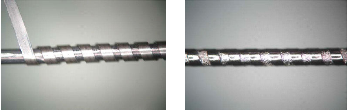
Figure 3.33 - Picture showing the copper ribbon spirals, the high-lead solder and column after wave soldering [Winslow 2005]
