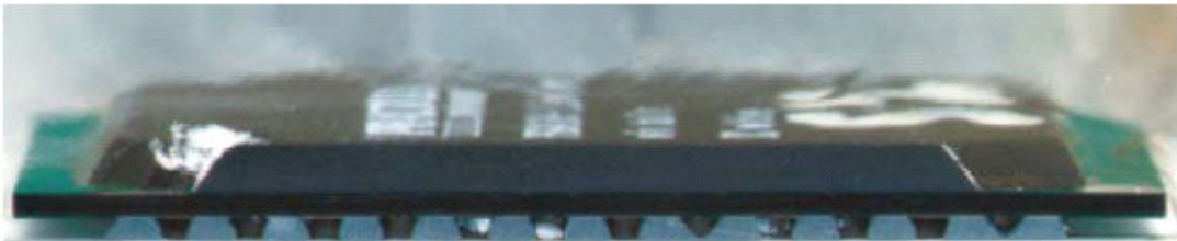
Figure 3.27 - Cross-sectional view of plastic package with Microperl-SOL and conventional solder ball [Sekisui 2005]
