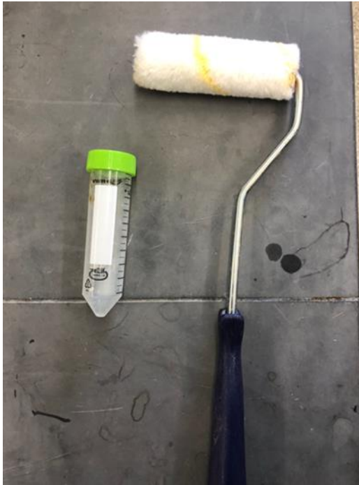
Figure 3.4: Photograph of the Roller Swab attached to the roller handle for sampling
