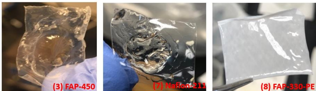
Figure 5.4. Photographs of peeled membranes after resistance measurements.
