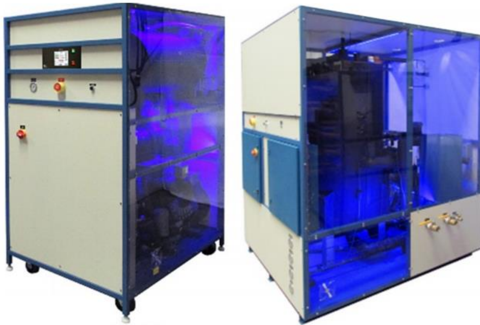
Fig. 11: Chiller with up to 25 kW of cooling power (left) and pump module with three dedicated pumps and in line and immersion heaters (right)
