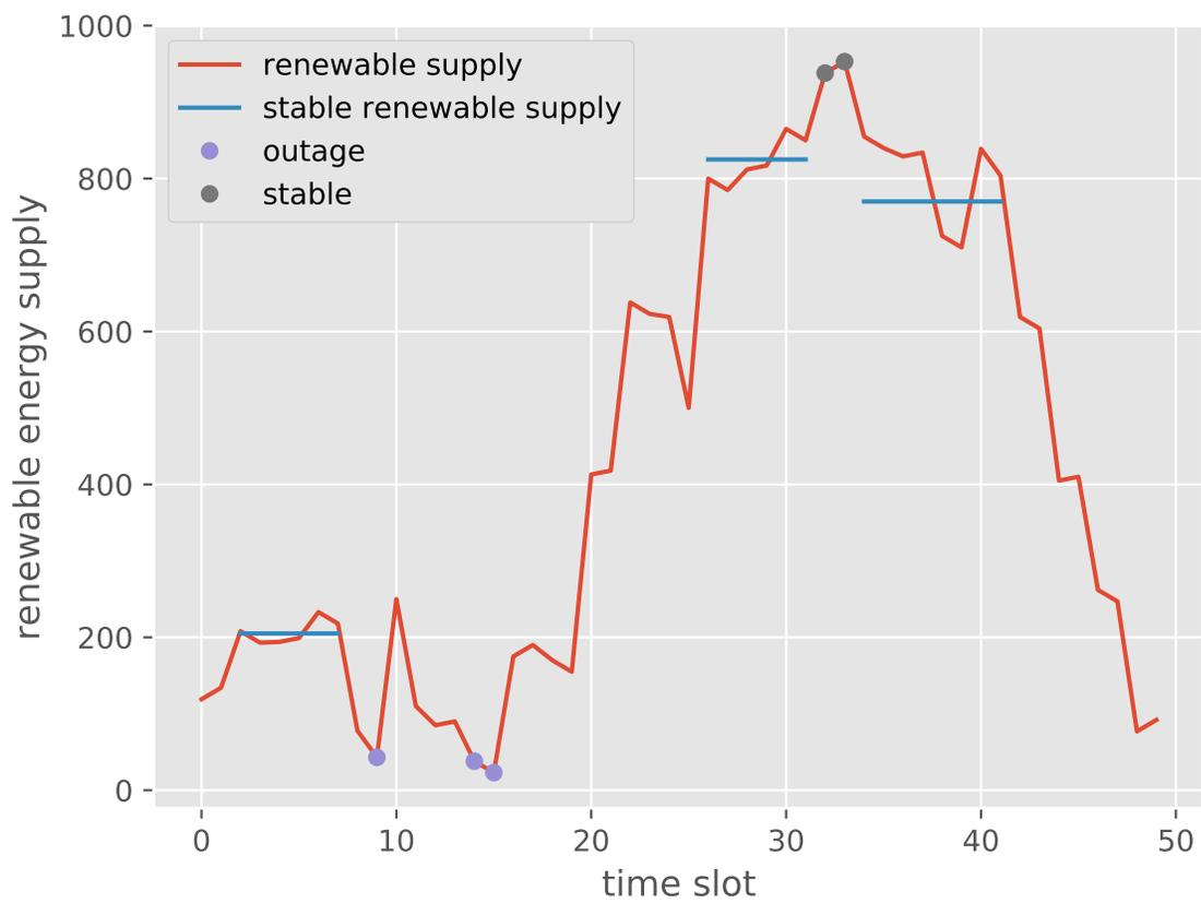
Figure 5.2: An example of the three state cases (i.e., *OTA*, *STA*, and *FLU*) of renewable energy supplies. The unannotated values are defined as fluctuate states or *FLU*.
