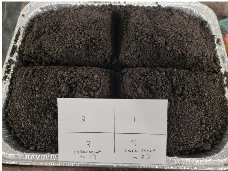
**Figure 14:** Quartered Specimen with Companion Samples Indicated
