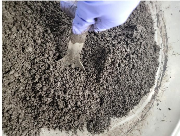
**Figure 12:** Slurry Surfacing System Mixed to Crumble
