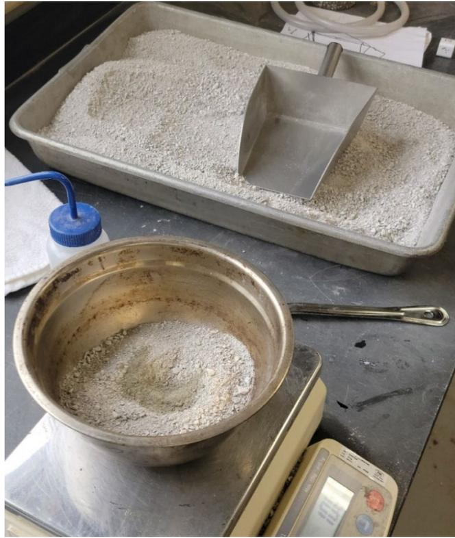
**Figure 6:** Sample Mixing with Aggregate and Mineral Filler
