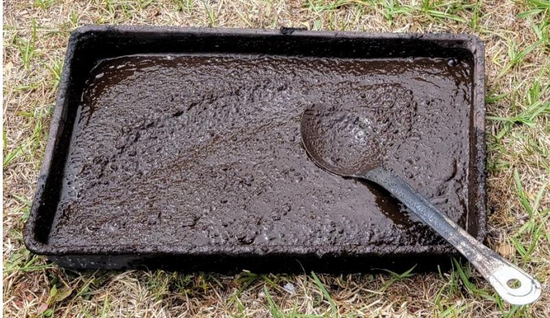
**Figure 13:** Field Sampling Rigid Pan with Breaking Mixture
