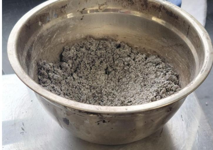
**Figure 7:** Aggregate, Mineral Filler, and Water Mixed
