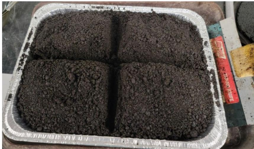
**Figure 11:** Mixed to Crumble Quartered Sample with Taping Knife
