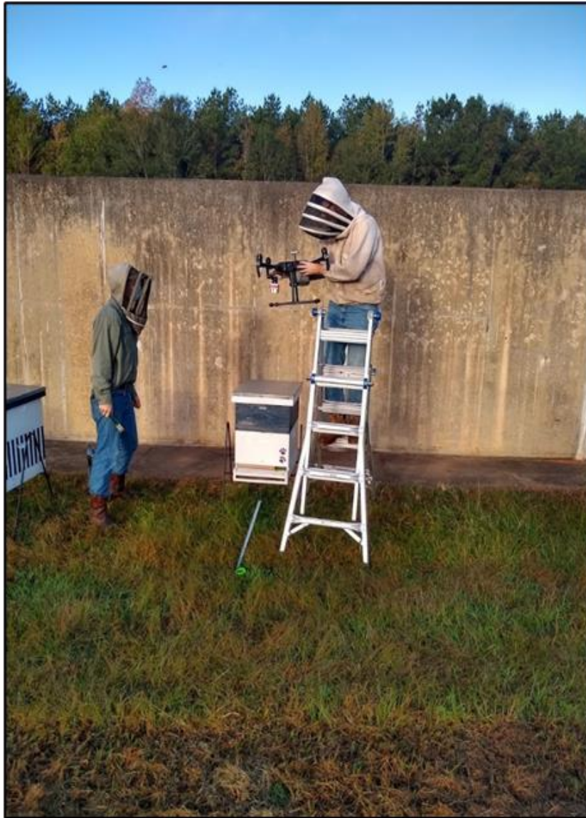
Figure 3.1 Thermal image capture of a honey bee ( Apis mellifera ) colony from above with inner and outer lids in place. Thermal images were captured with a DJI Matrice 200 V2 drone equipped with a Micasense Altum thermal sensor. The thermal image taken here was from above with the inner and outer lids in place.
