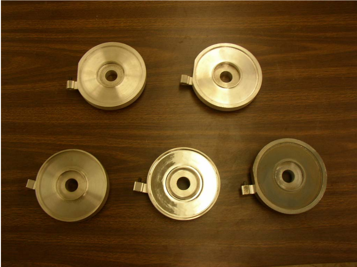
Figure D.5 Wall friction samples (Top row, left to right: milled aluminum, mirror finished aluminum; Bottom row, left to right: milled steel, mirror finished steel, and carbon coated steel)
