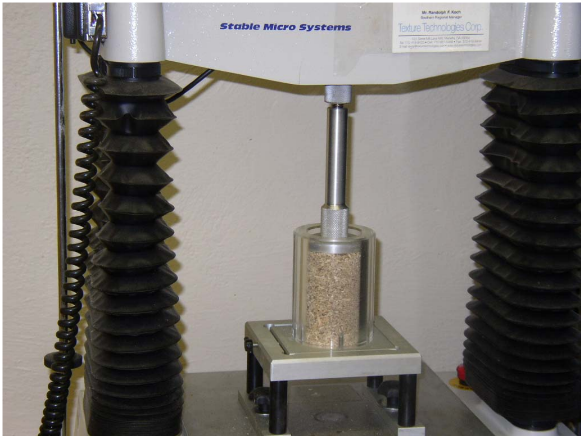
Figure D.1 Texture analyzer with compression cell and tight fitted piston
