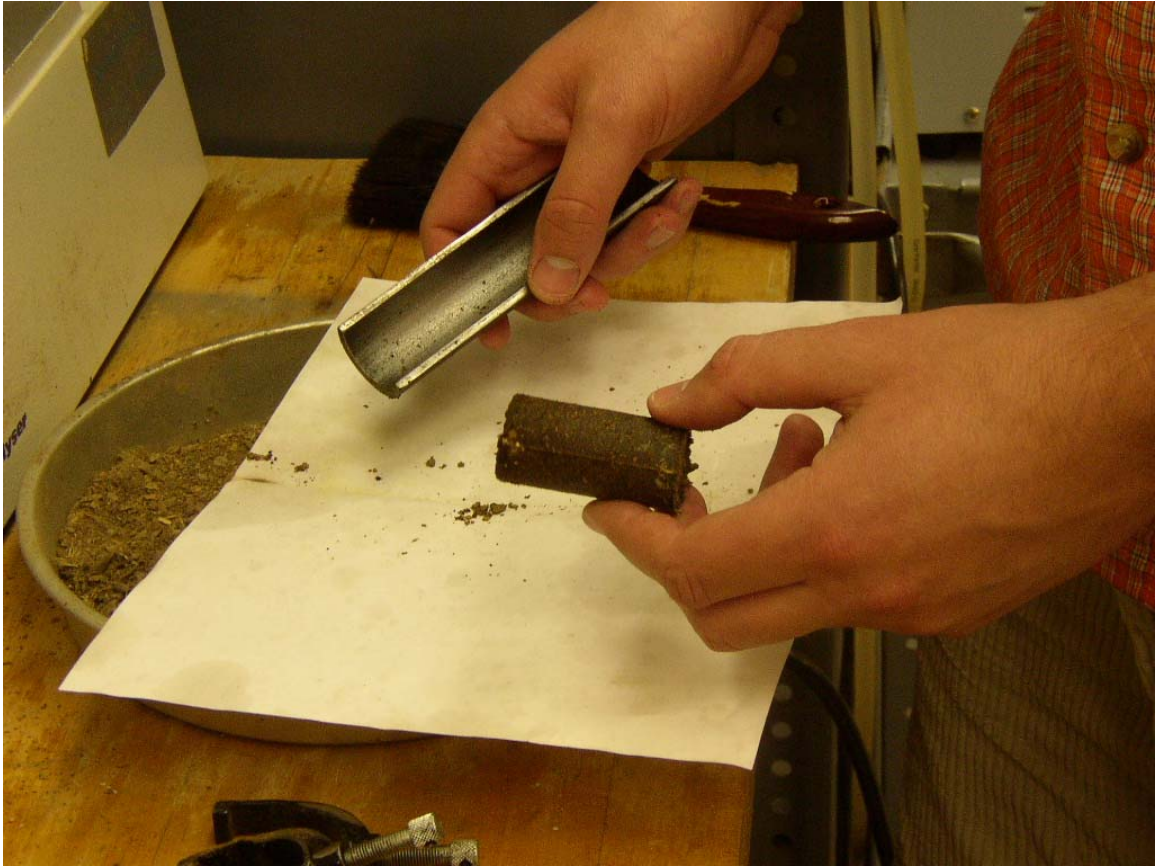
Figure D.3 Poultry litter compact removed from compaction die
