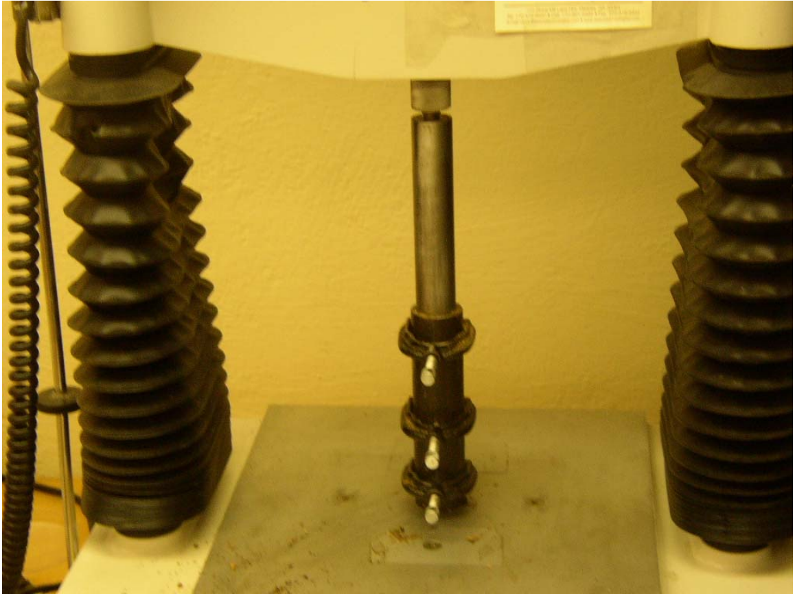
Figure D.2 Clamped compaction die filled with poultry litter below a plunger attached to the crosshead of the texture analyzer before compaction
