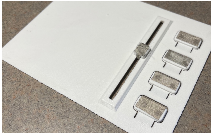
Figure 71: Type 3 3d printed model wrapped with conductive fabric
