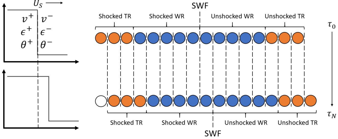
Figure 3.2: Mechanism of the atomistic moving window technique.
