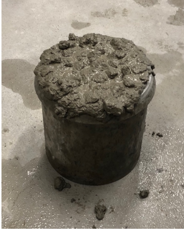
Figure 3-5: Preparation for Unit Weight Test
