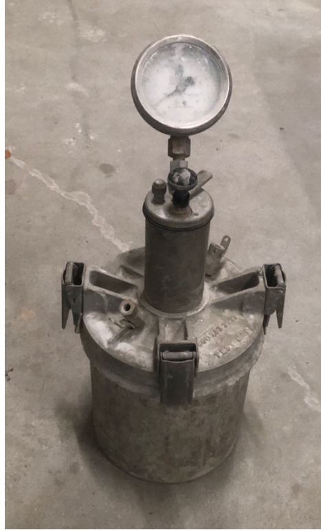
Figure 3-6: Air Content Test
