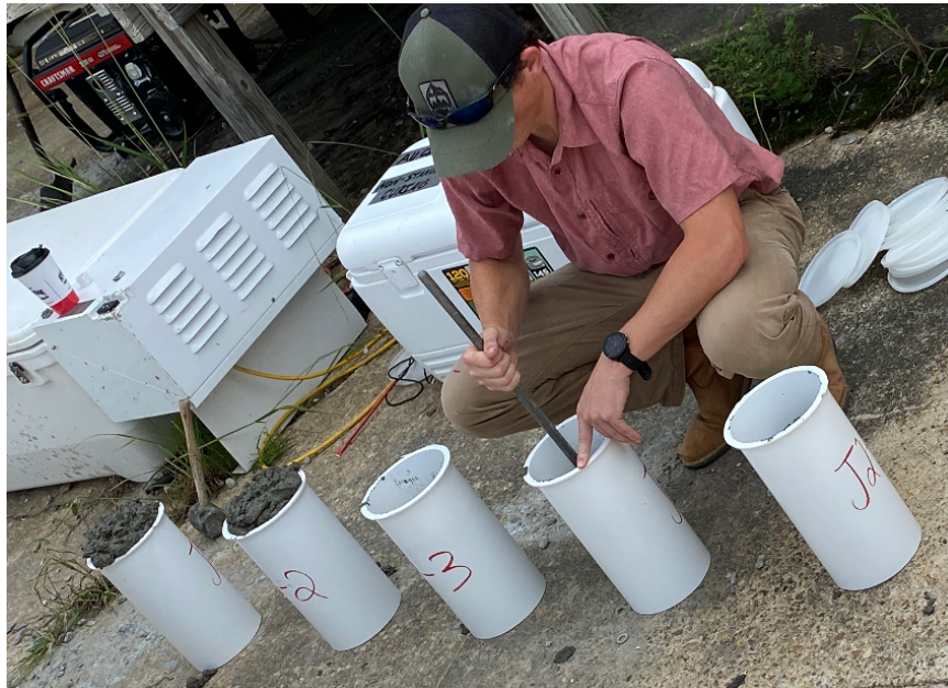
Figure 1-1: Concrete cylinders being prepared for initial curing
