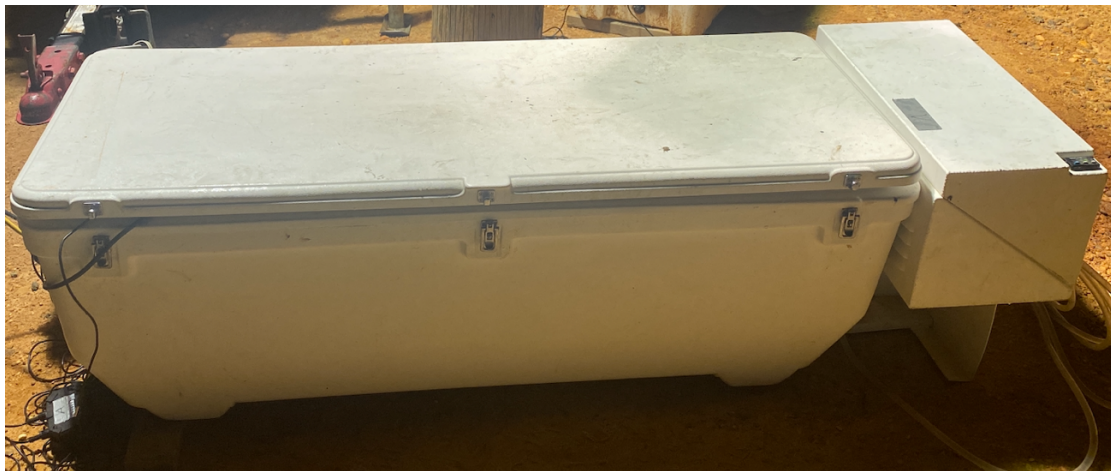
Figure 1-2: Initial curing box used at the jobsite
