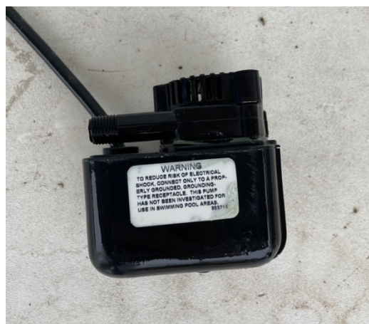
Figure 3-11: Submersible Circulation Pump
