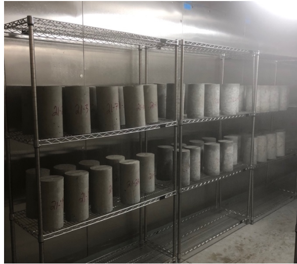
Figure 3-14: Cylinders in Final Curing Room
