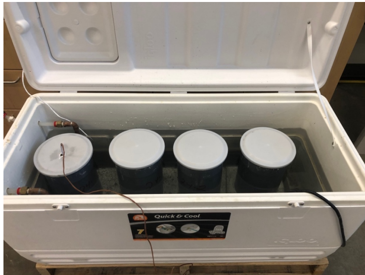
Figure 3-12: Cylinders in Initial Curing Tank
