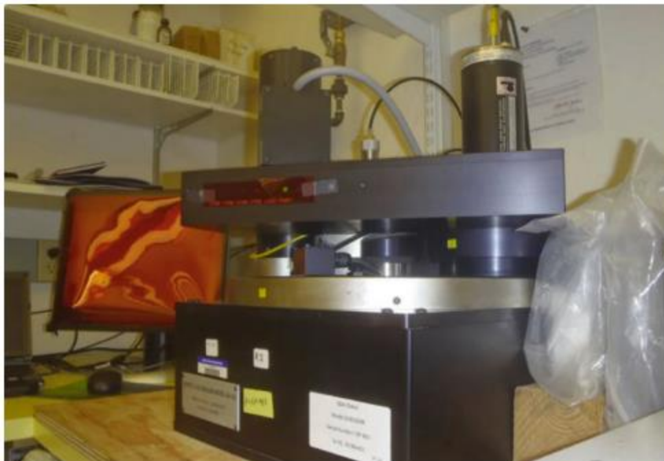
Figure 3.3: DA-20 Risø TL/OSL Reader at the E.L. Cord Luminescence Laboratory at Desert Research Institute (From Keen-Zebert, 2013)
