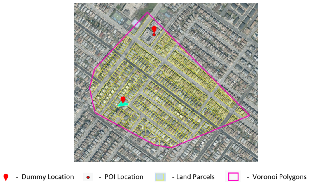
Figure 5.4: Voronoi parcel similar to v_{true} from cosine similarity search, residential parcel prclSim_1 similar to p_{true} from Euclidean similarity search and the two dummies ( dummy_{residential} and dummy_{poi} ) identified.
