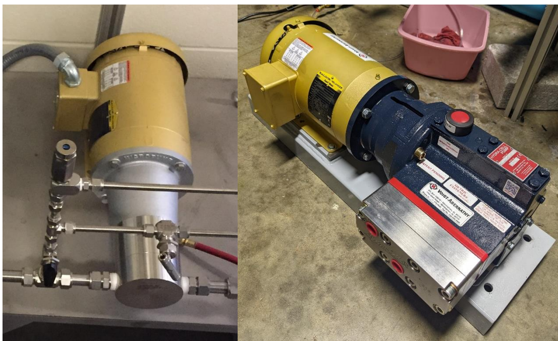
Figure 3.15: Refrigerant gear pump (left) and refrigerant diaphragm pump (right)
