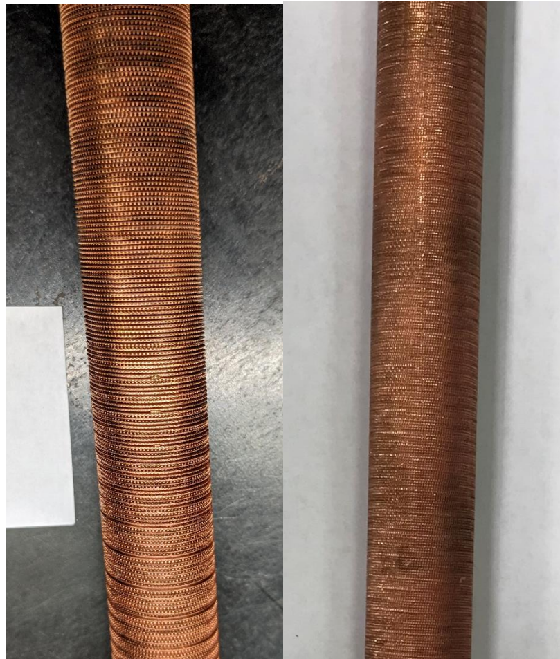
Figure 3.6: Tube-C condensing surface (left) and Tube-B evaporation surface (right)
