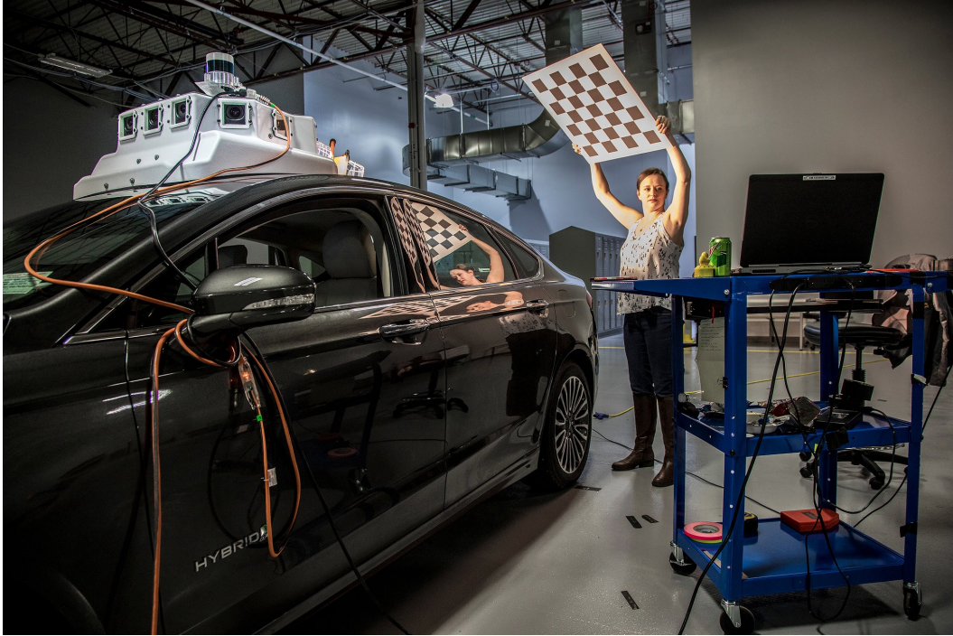
Figure 1.1: A manual calibration takes place in front of a calibration target [73].
