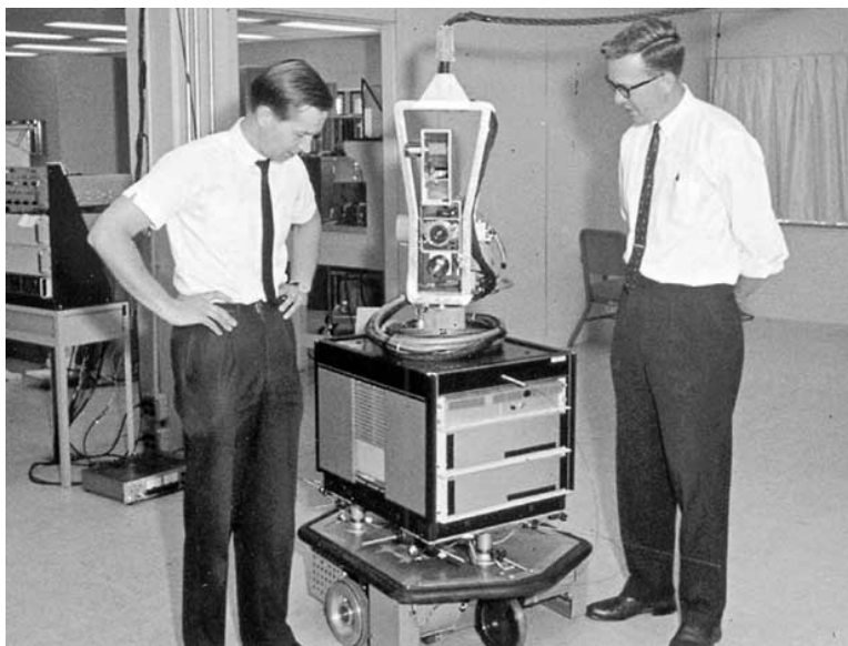
Figure 1.2: 'Shakey' was an early attempt at an autonomous mobile robot [19].
