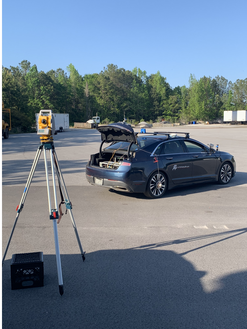
Figure 7.1: Experimental setup. The surveying tool (at left) was used to capture the ground truth sensor positions and orientations.
