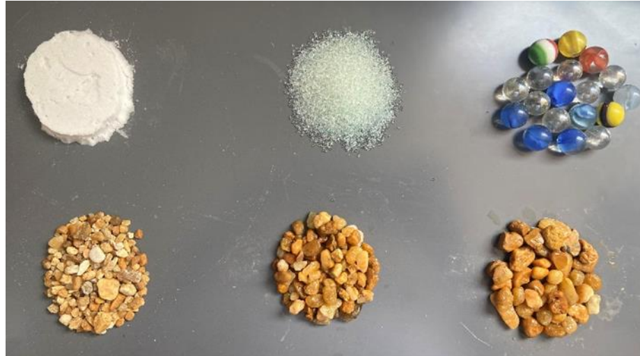
Figure 3.6: Tested porous media materials.
