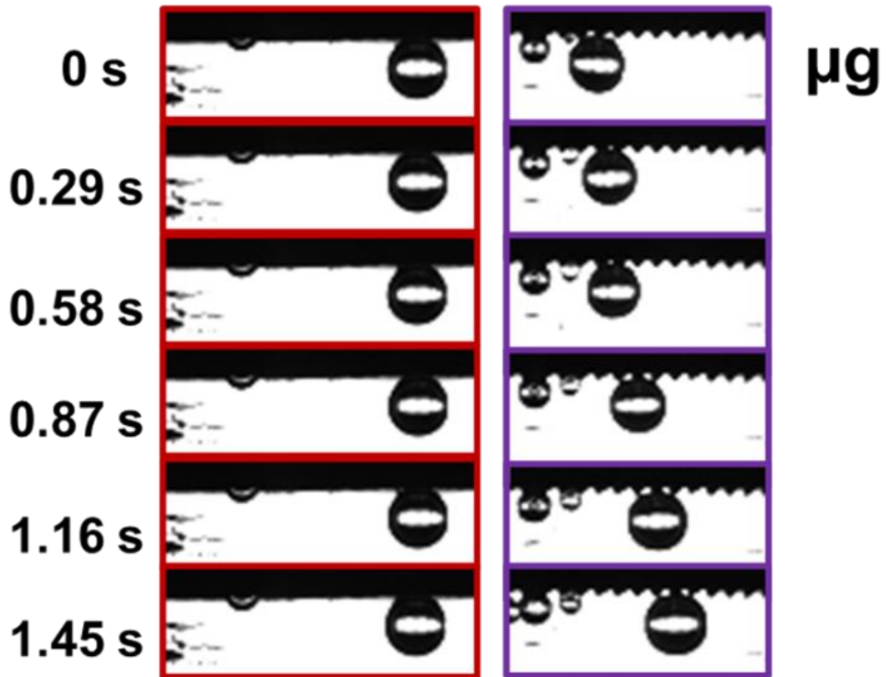
Figure 4.15 Comparison of vapor bubble dynamics from the flat baseline surface (left) and the 60°-30° microstructure (right) at 0.50 W/cm 2 . The 250 μm square cavities produce consistent nucleation activity on both test surfaces, but vapor bubbles ride on the crests of the sawteeth at the departure diameter.
