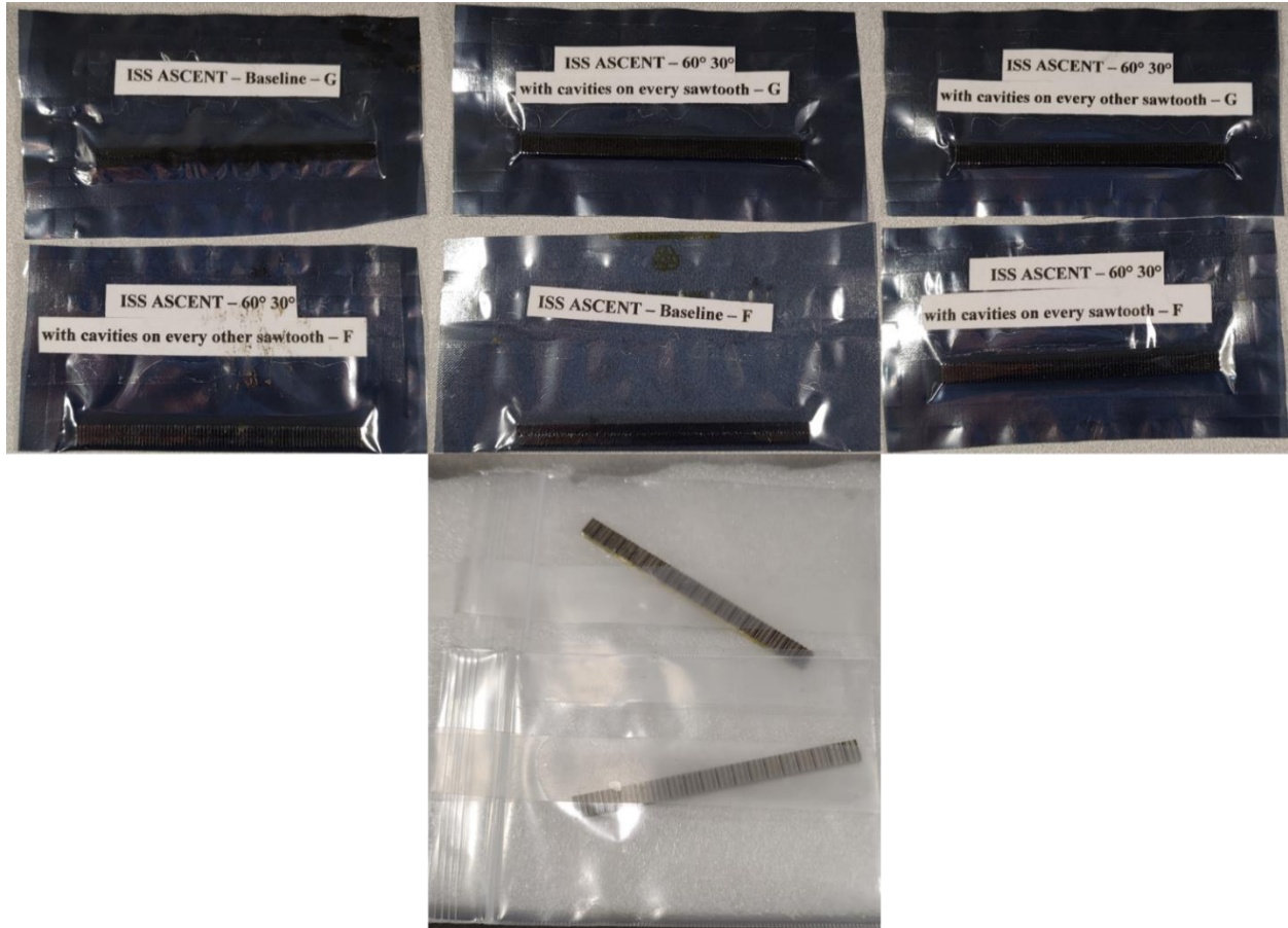
Figure 2.7 The final test surfaces shipped from Auburn University and the University of California, Davis. The vacuum-sealed packages from Auburn University are illustrated at the top, and the two wire EDM test surfaces from the University of California, Davis, are shown at the bottom. The Auburn University test surface with the trailing label "-F" indicates a flight surface, and "-G" denotes a ground surface.
