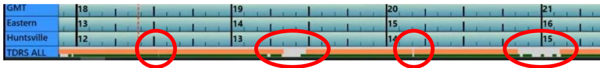
Figure 4.3 The ISS flight plan indicating loss-of-signal period due to satellite handovers and line-of-sight constraints within the Tracking and Data Relay Satellite System. The orange and green bar indicate the availability of different feeds (video, voice, data etc).
