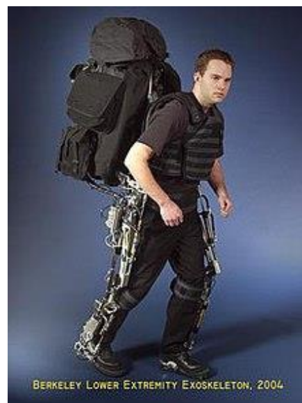
Figure 4; BLEEX hydraulic exoskeleton prototype being used for carrying a load [7]
