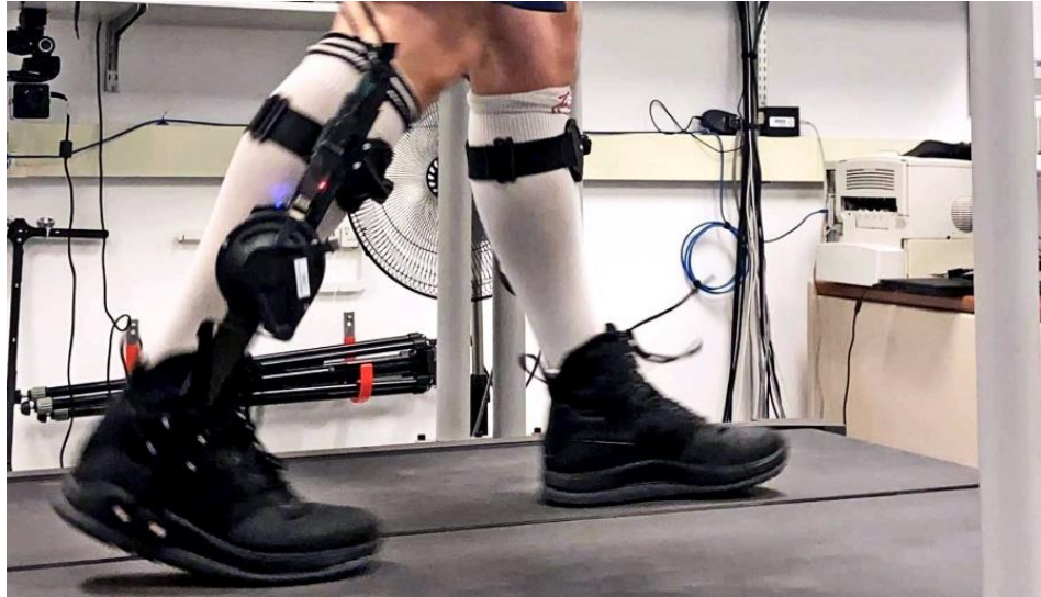
Figure 5; Electric motor actuated ankle exoskeleton used for reducing the metabolic cost of walking [26]
