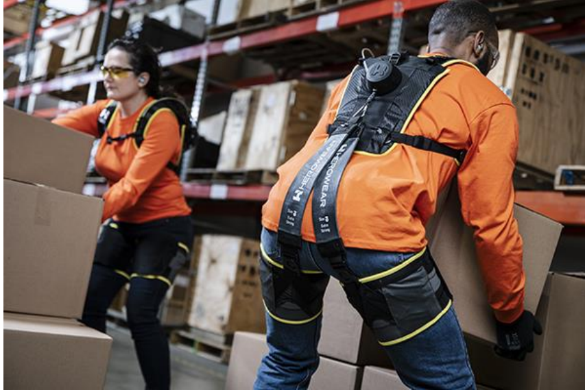
Figure 2; Herowear exoskeletons being used to assist lifting [11]
