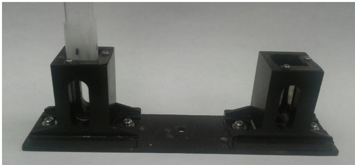
Figure 4.1: Setup for solution and swollen films utilizing glass test tubes sealed with rubber septa placed in a Shimadzu UV/Vis holder.
