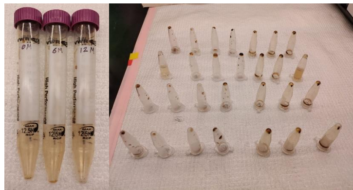
Figure 0.2. CELF Lignin particle production, evidence of complete solubilization of lignin (left). THF-salt solution ratio dissolution test (right).
