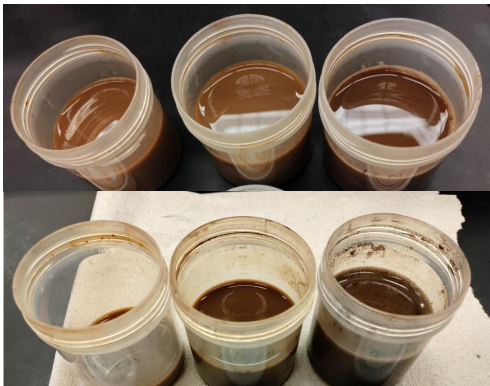
Figure 0.3. CELF Lignin particle production, stability over time. Initial production (top) and the same samples after 5 months of storage in room temperature conditions (bottom).
