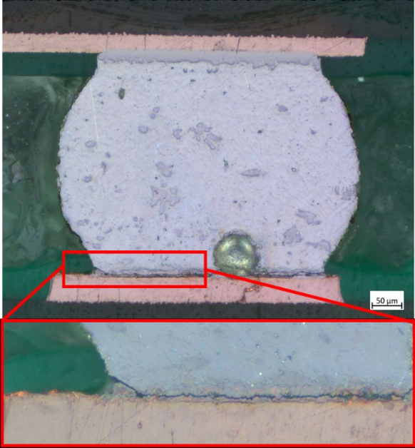
(b) 50°C – IMC layer failure
