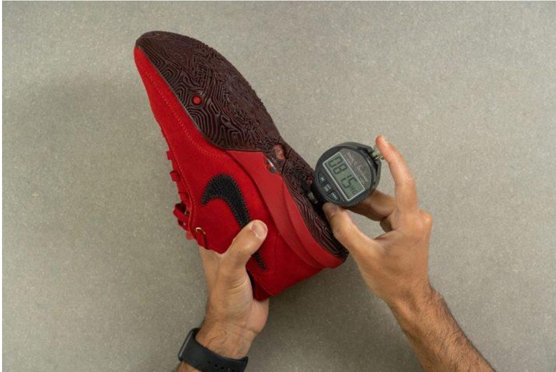
Figure 3.9 Curcic, D. (2023), Sole Softness Test. [Photograph]
