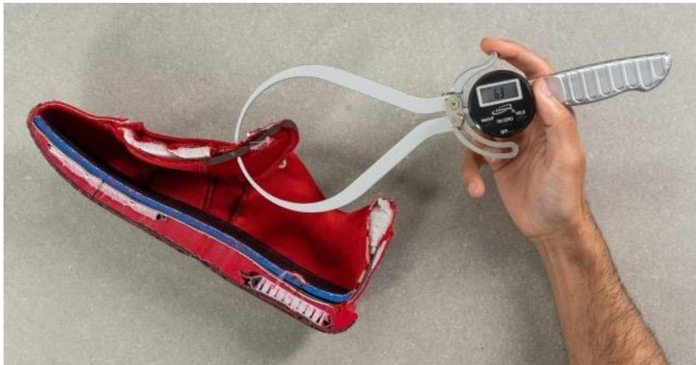
Figure 3.6 Curcic, D. (2023), Tongue Padding Thickness Test. [Photograph]
