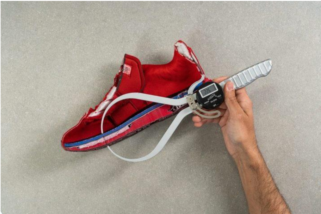
Figure 3.8 Curcic, D. (2023), Forefoot Stack Test (Average thickness of forefoot part).
