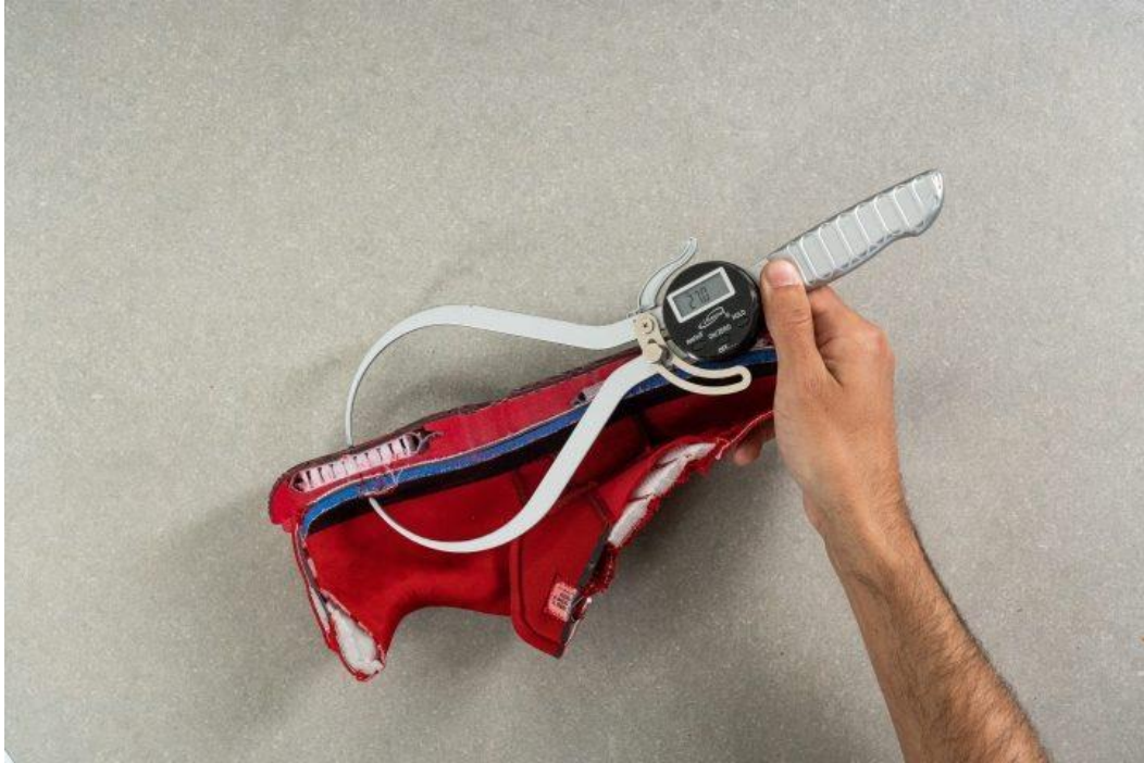
Figure 3.7 Curcic, D. (2023), Heel Stack Test (Average thickness of shoe heel part) [Photograph]
