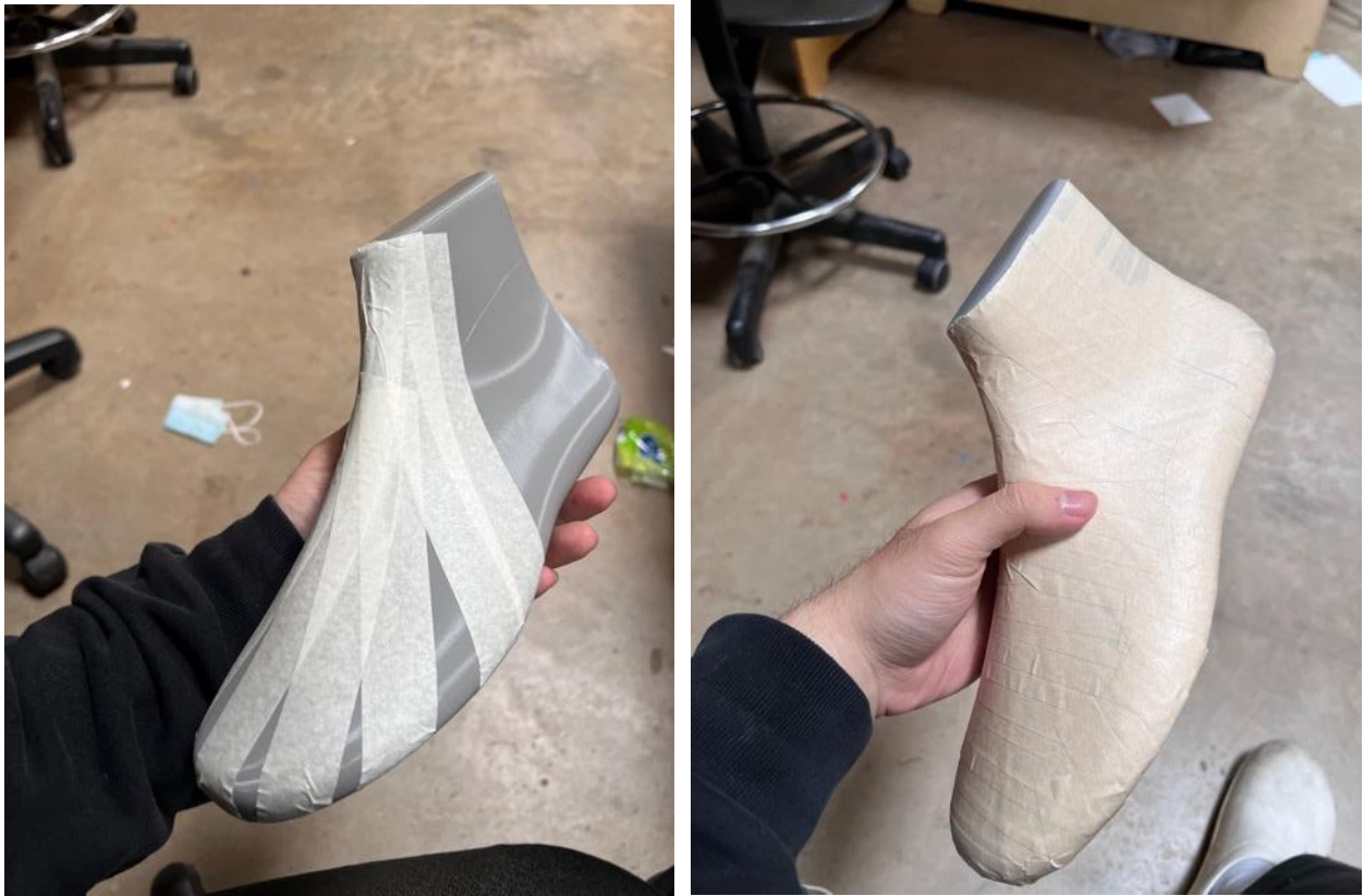
Figure 5.16 Taping shoe last
