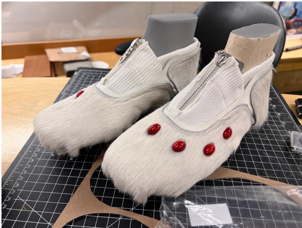
Figure 5.20 Fixing the upper shape.
